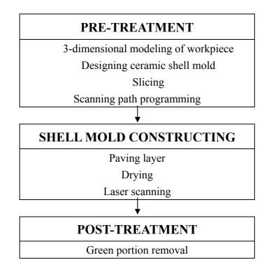
Fig. 3 The flow chart of ceramic shell mold fabricated by CLF
