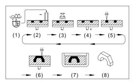
Fig. 1 CLF layer manufacturing flow diagram [9]
