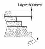
Fig. 2 The step effect and rough surface were formed by layer manufacturing in a 45 ° inclined plane
