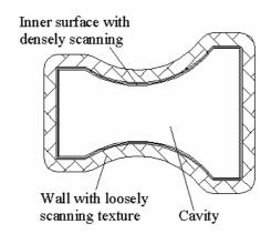
Fig. 4 Schematic of a ceramic shell mold made by CLF
