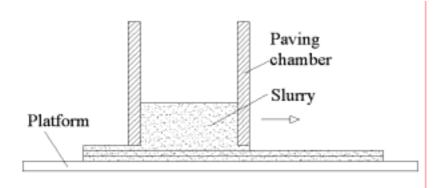
Fig 5 Schematic of CLF paving device
