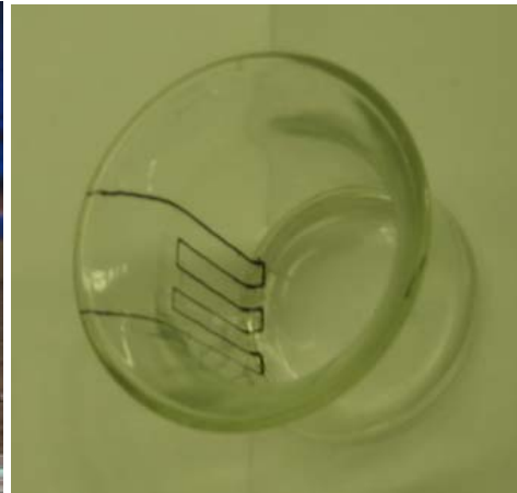
Figure 13 (a) The cup was fixed on the 2-D motion table; (b) Antenna pattern was printed on the 3-D inner surface of bugle cup with CIJ printing.
