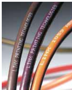
Figure 2 Three-dimensional pigmented CIJ printing in coding and marking (resource: www.linx.co.uk )
