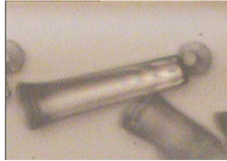
Figure 2 : Negative photoresist towers.
