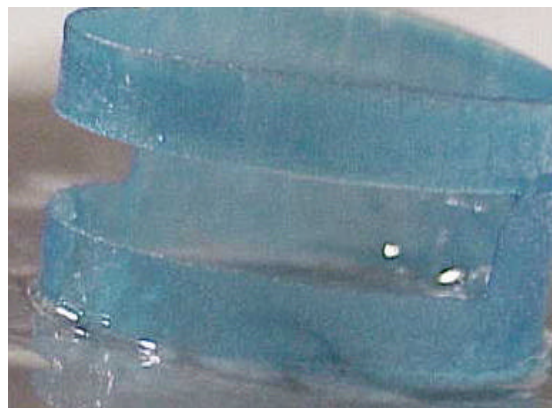
Figure 6: Ice part built with local cooling during interface layers
