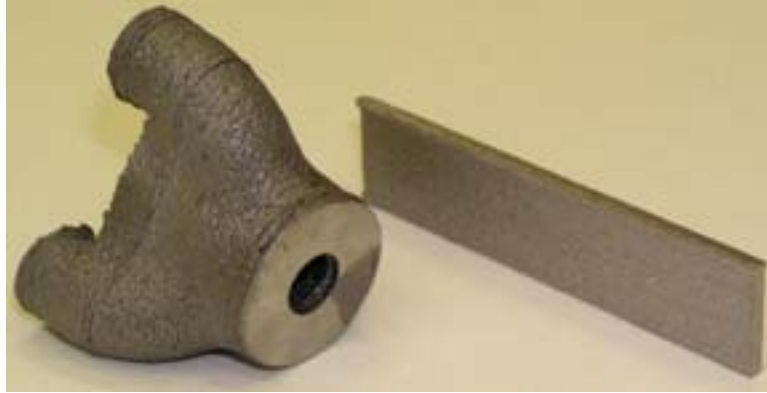
Figure 3 - Bulky (L) and Thin Walled (R) Parts
