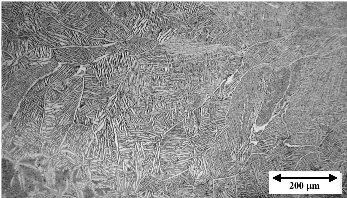
Figure 4 - Thin-Walled Microstructure at 100X Magnification
