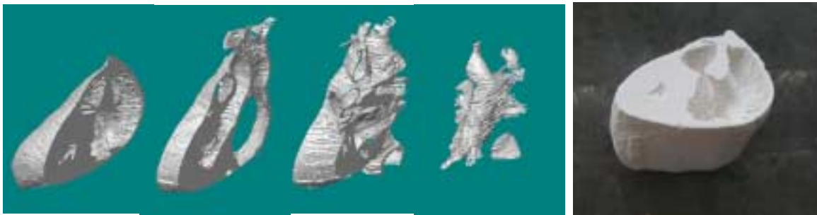
Figure 6. Left: Exploded view of four sections. Right: Expandable pattern
