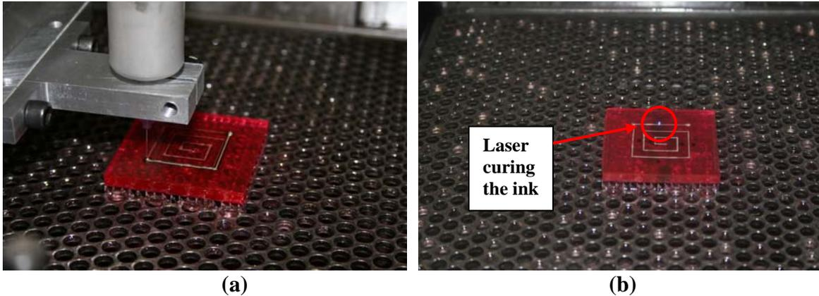
**Figure 7. (a) The direct write process, (b) laser curing of the conductive ink.**
