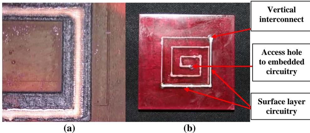
**Figure 8. (a) Image of the cured ink, (b) finished part.**
