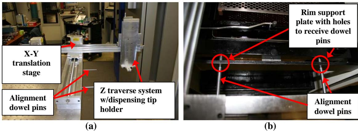
**Figure 2. (a) The 3-axes traverse system, (b) alignment of the SL/DW system.**
