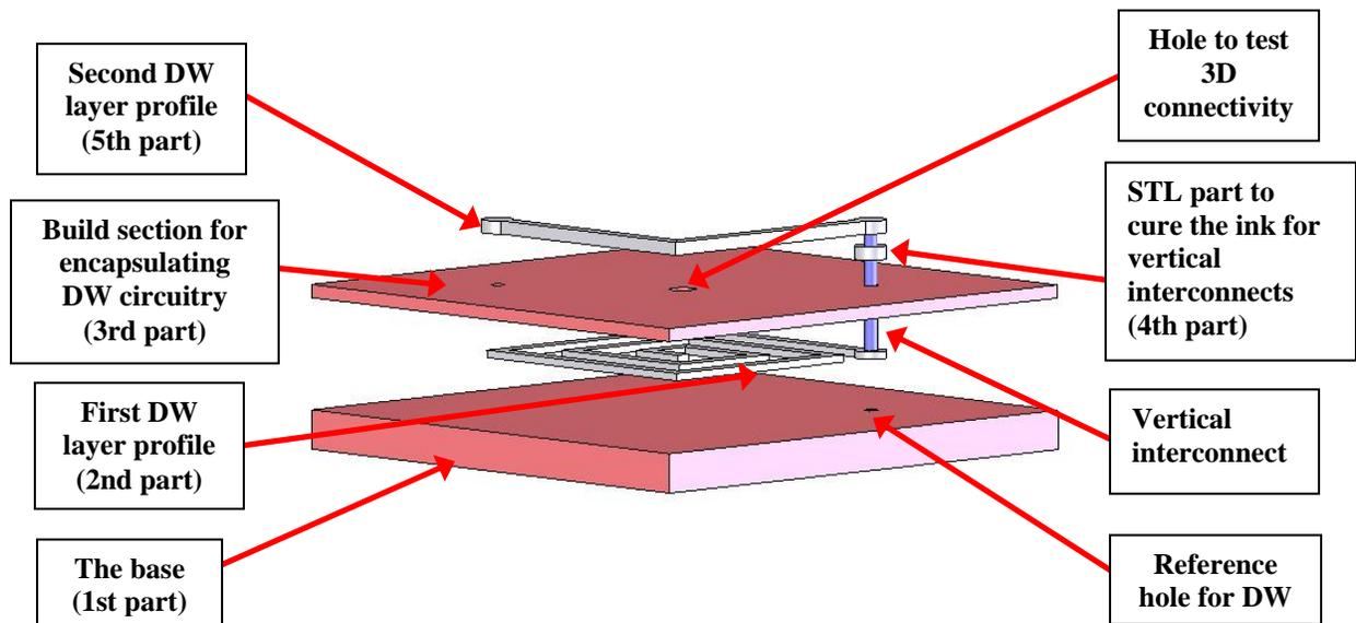
Figure 5. The hybrid SL/DW operation.
