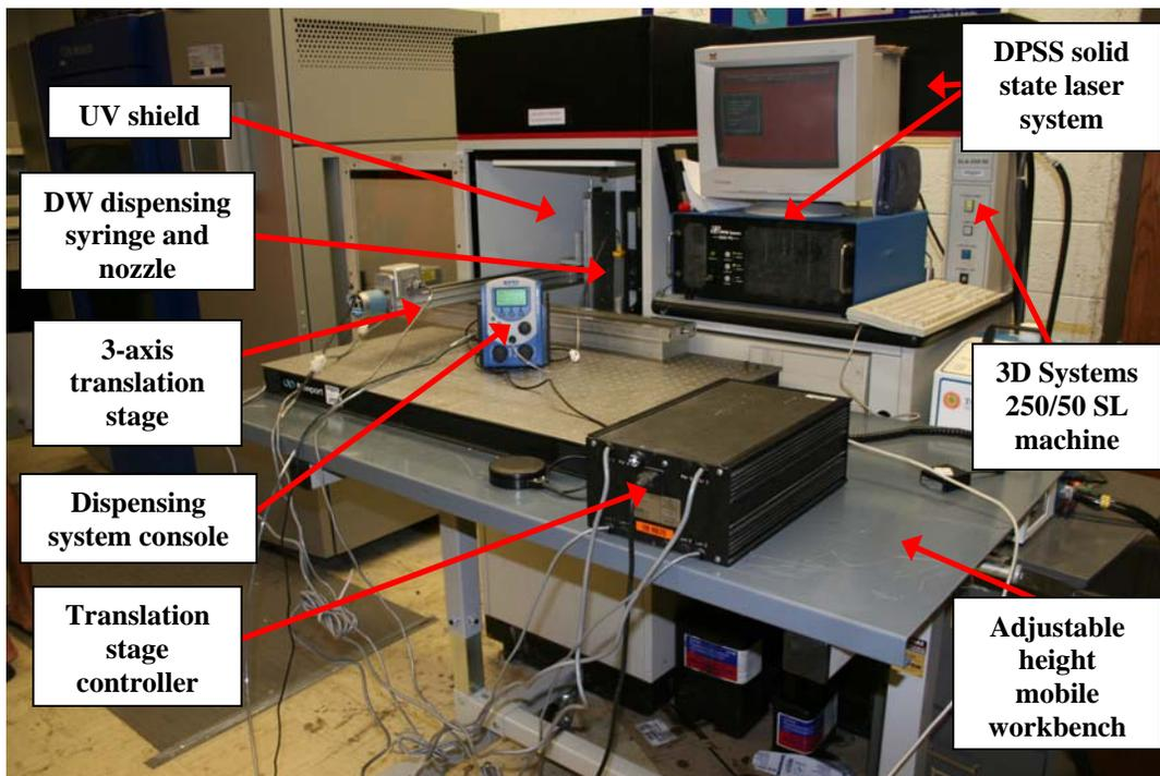
Figure 1. The hybrid SL/DW machine setup.
