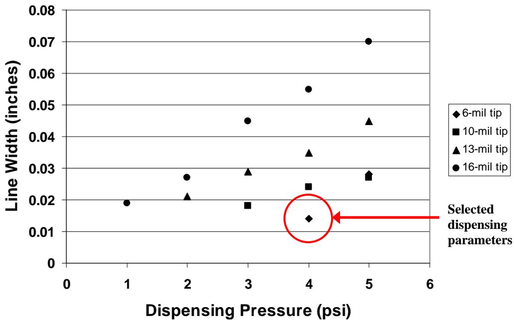
**Figure 4. Line width versus dispensing pressure for different size injection tips (0.0625 in/sec traverse speed and 5-mil distance between tip and surface).**
