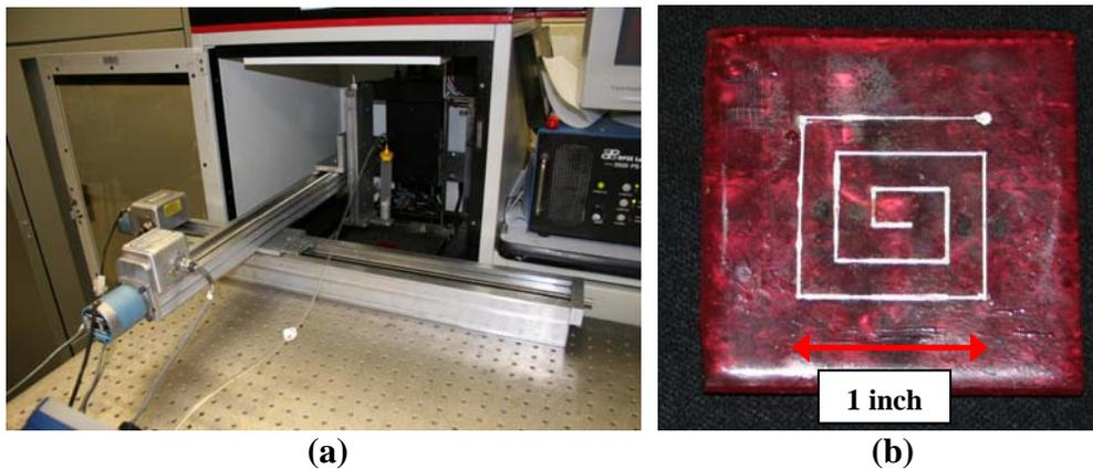
Figure 6. (a) The traverse system for DW, (b) DW circuit profile
