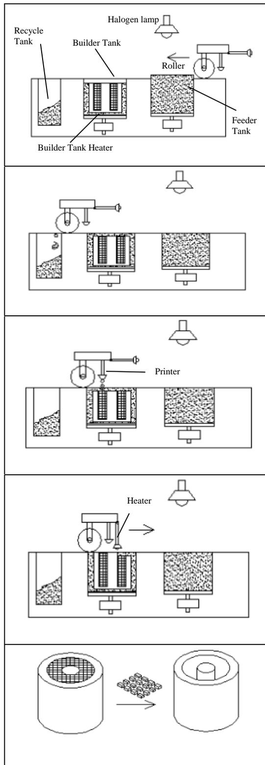
Figure 1. Selective Inhibition Sintering process steps
