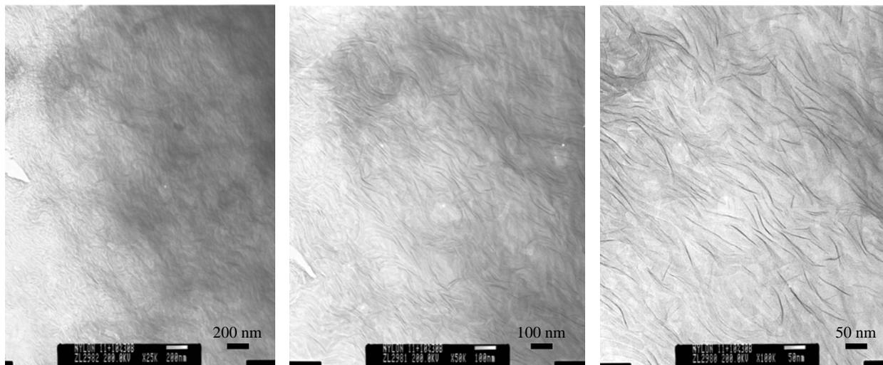
**Figure 1** TEM micrographs of the 90% PA11:10% Cloisite 30B polymer showing exfoliation of nanoclay in PA11 was achieved.
