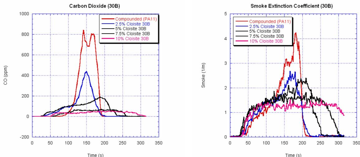
**Figure 6 and 7** Comparison of carbon monoxide yield (left) and smoke extinction coefficient (right) for 2.5, 5, 7.5, 10 wt% of Cloisite® 30B PA11N at 50 kW/m<sup>2</sup> heat flux.
