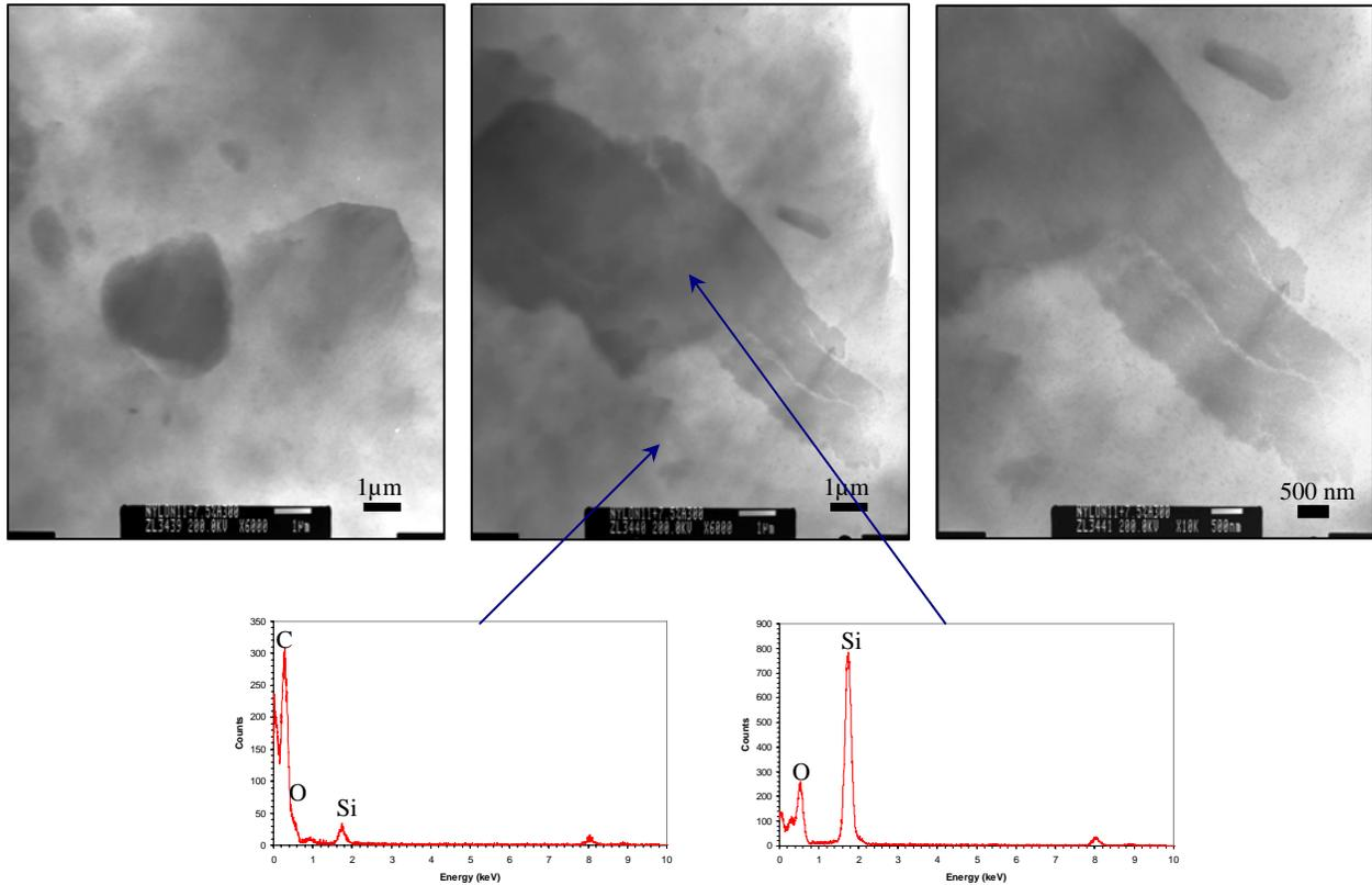
**Figure 3** TEM micrographs of the 92.5% PA11:7.5% Aerosil® 300 nanosilica polymer showing very large nanosilica aggregates were formed in the PA11 polymer.
