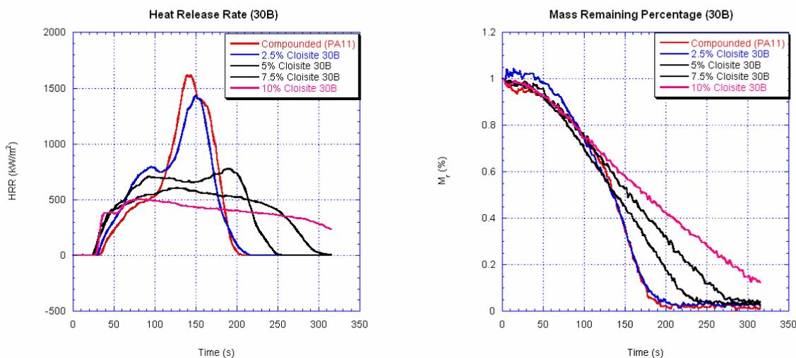
**Figures 4 and 5** Comparison of heat release rate (left) and residue mass (right) for 2.5, 5, 7.5, 10 wt% of Cloisite® 30B PA11N at  $50 \text{ kW/m}^2$  heat flux.
