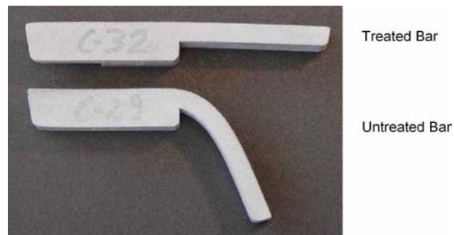
Figure 2 Photo comparing the deflection of 410 stainless steel bars with and without nanoiron treatment. The treated bar received four applications and was dried under a magnetic field. Both bars were deflected without prior sintering except the 1000°C sintering required to create the initial geometry.
