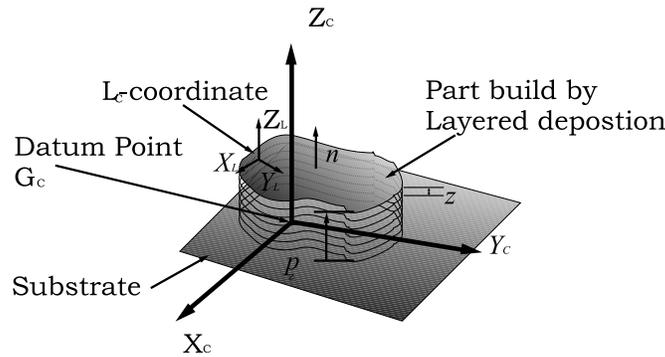
**Fig. 2.** The Coordinate Systems used in the Error Propagation Estimation
