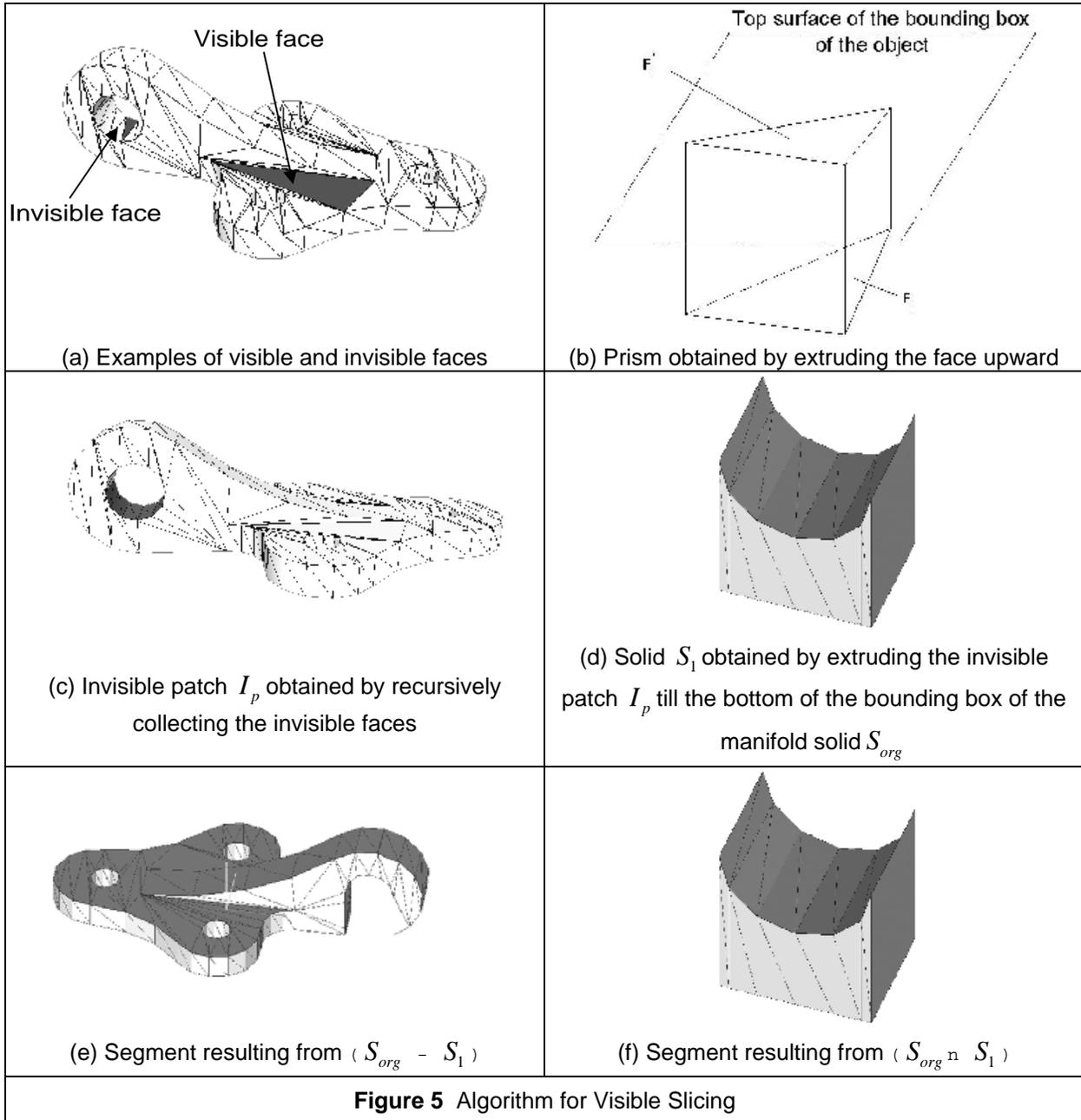
If the slicing is accurate enough, the horizontal surfaces of the object can be obtained during the slicing operation itself whereas the non-horizontal surfaces will require machining in scan milling. Therefore, after obtaining the set of visible slices that have the least heights, the authors prefer to split them further if any of the slices have large horizontal surfaces. Accordingly, the
