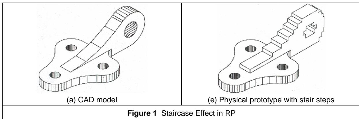
**Figure 1** Staircase Effect in RP
