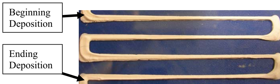
Figure 2: Deposition lines using constant ram velocity ( v = 0.5 \mu\text{m/s} ). Table speed is 25 mm/s and nozzle diameter is 580 \mu\text{m} .
