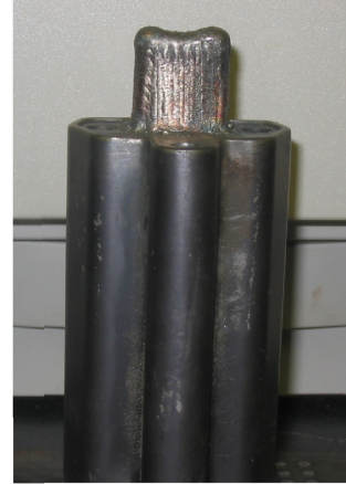
Figure 14. Repaired Core - via Automated Part Repair
