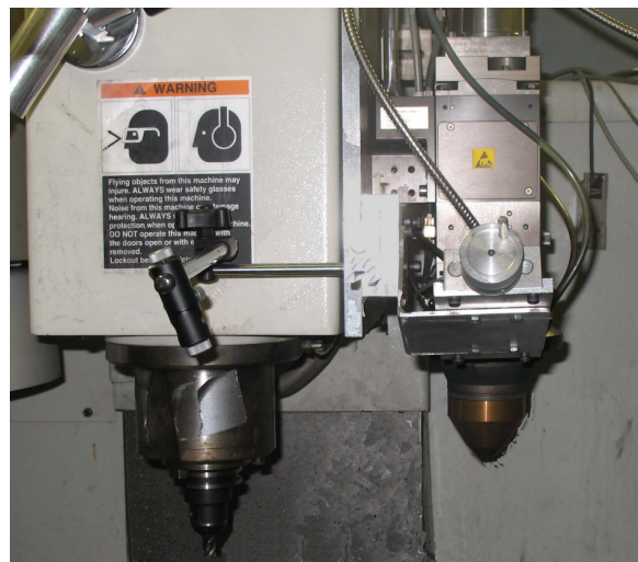
Figure 2. Integrated 5-axis FADAL CNC and Laser Deposition Head
