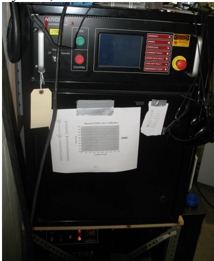
Figure 1. 1.0 KW Nuvonyx Diode Laser (808 nm wavelength)
