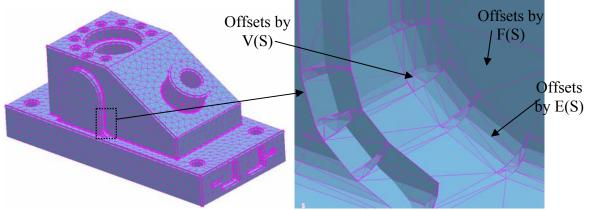
Figure 8: Candidate offsetting boundary for an input mesh.
