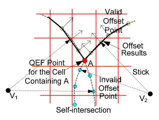
Figure 9: An illustration of our point-based offsetting method.
