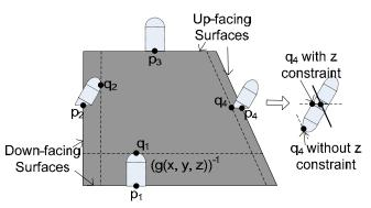
Figure 7: Different offsetting results for up-facing and down-facing triangles.
