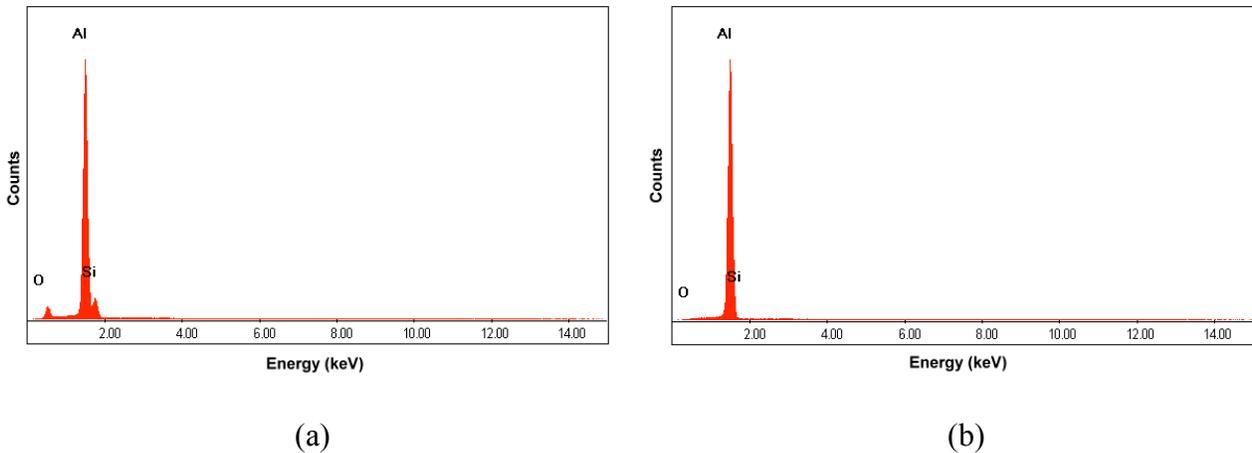
Fig.4. (a) EDS spectra showing a distinct oxygen peak in the thin layer with a different contrast. (b) The oxygen peak is absent in the regions adjacent to, but outside the thin layer.
