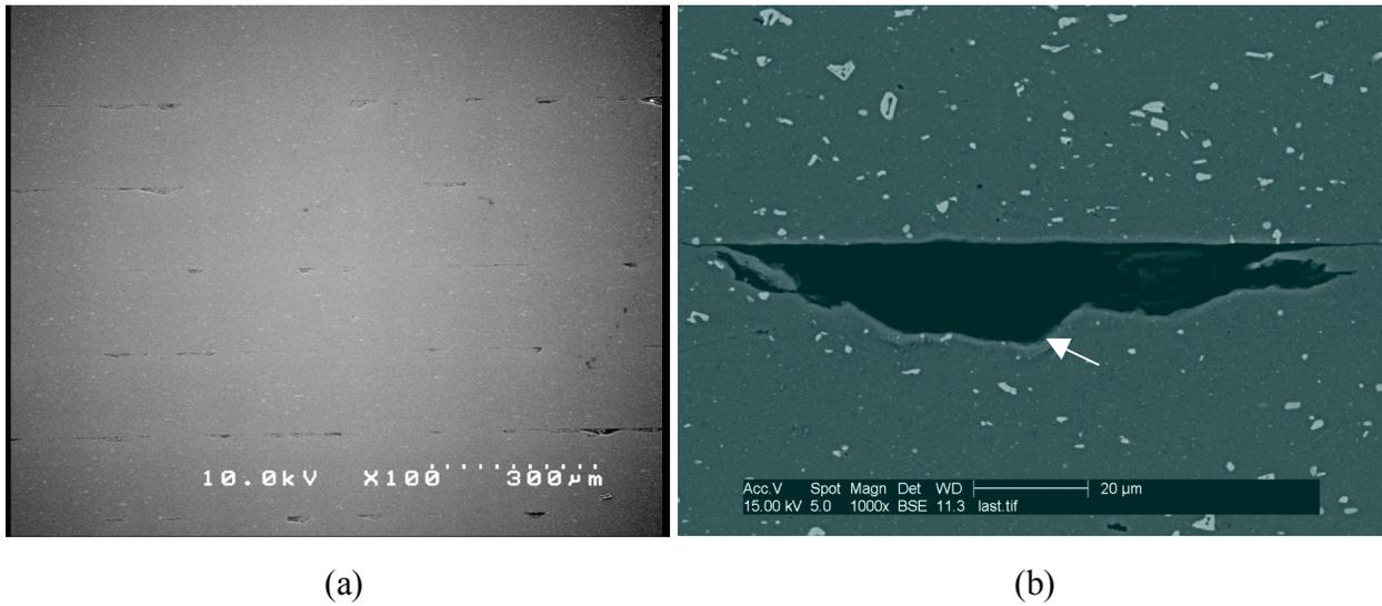
Fig.3. Defects/unbonded regions in ultrasonically consolidated Al 3003: (a) Low magnification, Secondary electron image; (b) High magnification, Back-scattered electron image (note the thin layer with a different contrast all around the defect (shown by arrow)).
