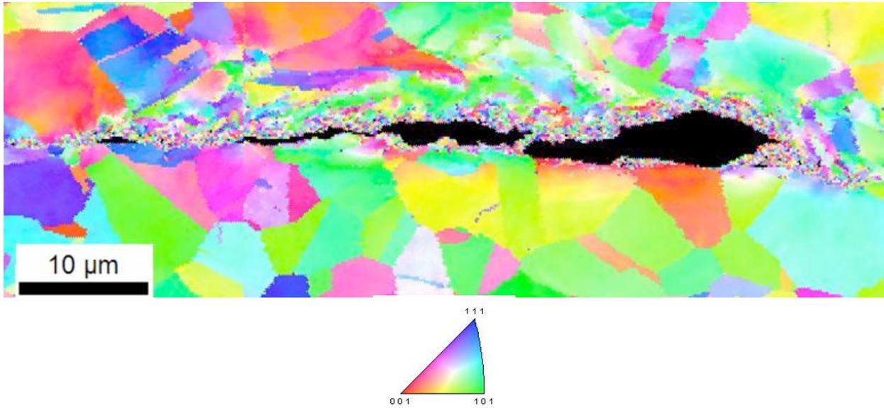
Fig.10. Inverse pole figure of an unconsolidated portion of the Ni-Ni interface. Note the extremely fine grains that are present along the defect boundaries.
