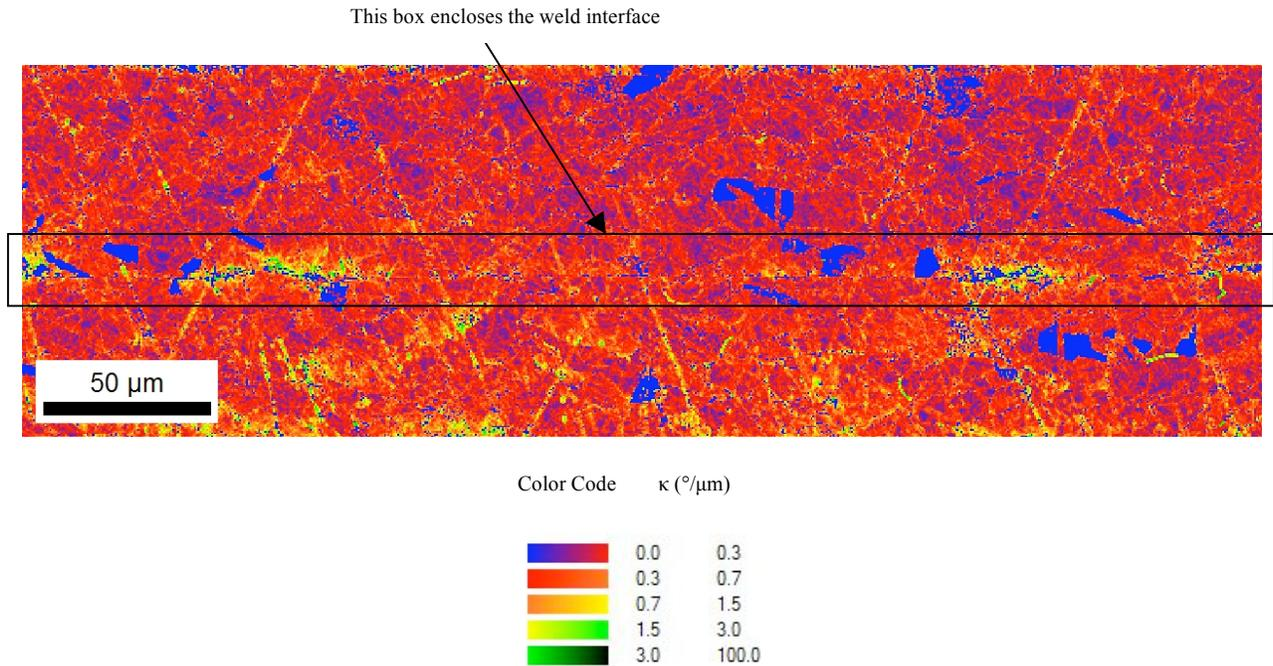
Fig.9. Average curvature map overlaying the SEM image of the ultrasonically consolidated Ni 201 layers.
