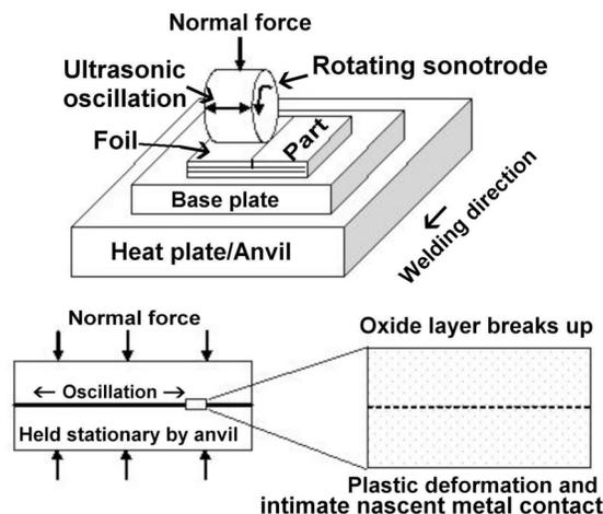
Fig.2. Schematic of the UC process.
