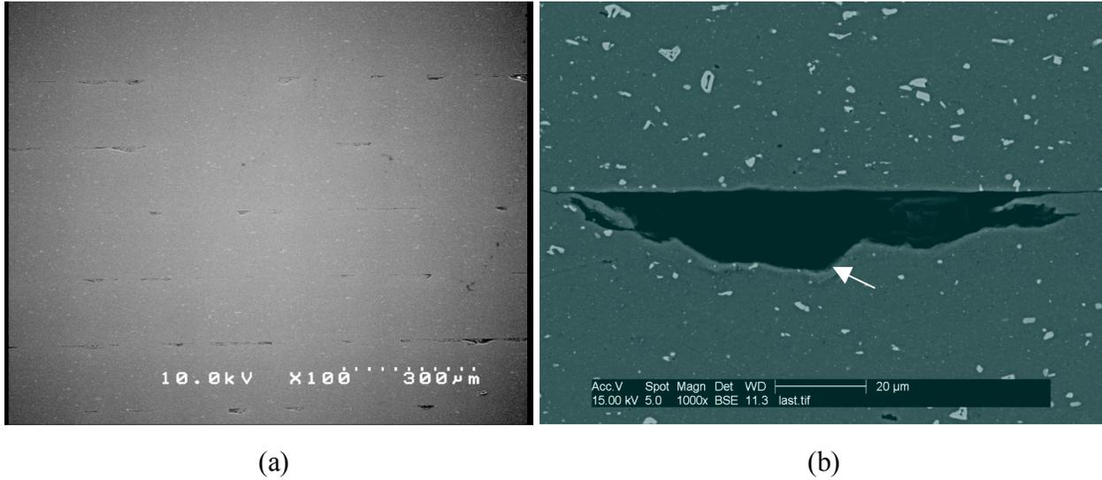
Fig.3. Defects/unbonded regions in ultrasonically consolidated Al 3003: (a) Low magnification, Secondary electron image; (b) High magnification, Back-scattered electron image (note the thin layer with a different contrast all around the defect (shown by arrow)).
