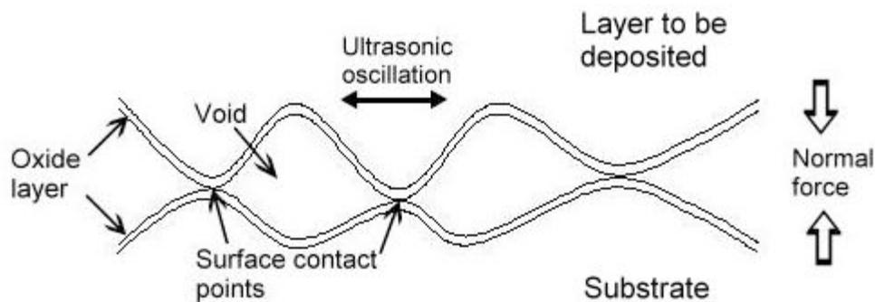
Fig.11. Schematic of the mating surfaces at the beginning of ultrasonic welding.
