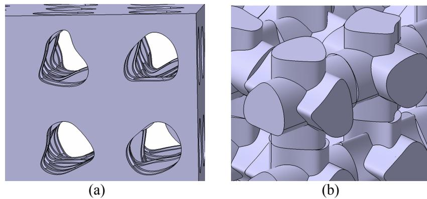
**Fig. 7** Case 2: More details of the step changes of the cross sections for: (a) scaffold, (b) theoretical regenerated bone.
