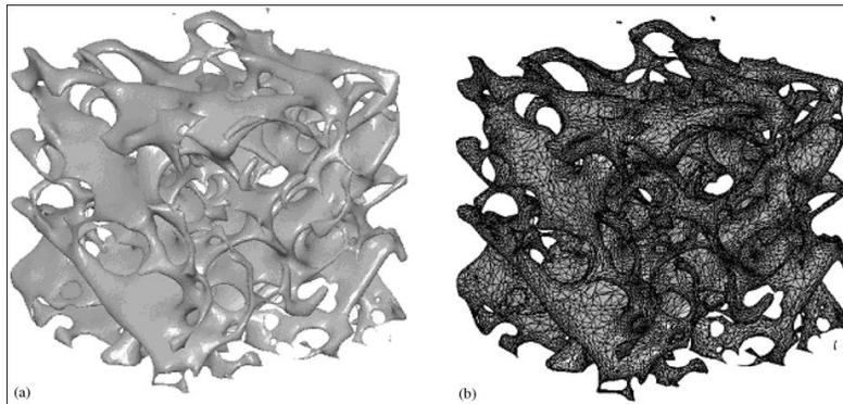
**Fig. 3** Volumetric rendering of a human trabecular bone from  $\mu$ CT (a) and STL representation for layer manufacturing fabrication (b) (Das *et al.*, 2003).
