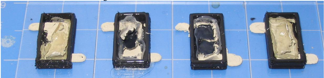
**Figure 5. Poor casting results for IPMC materials in (Design 1) relay housings constructed of GE Silicone II RTV, and electrical contact material SS26F; note the thick rims, curled and/or cracked surfaces**
