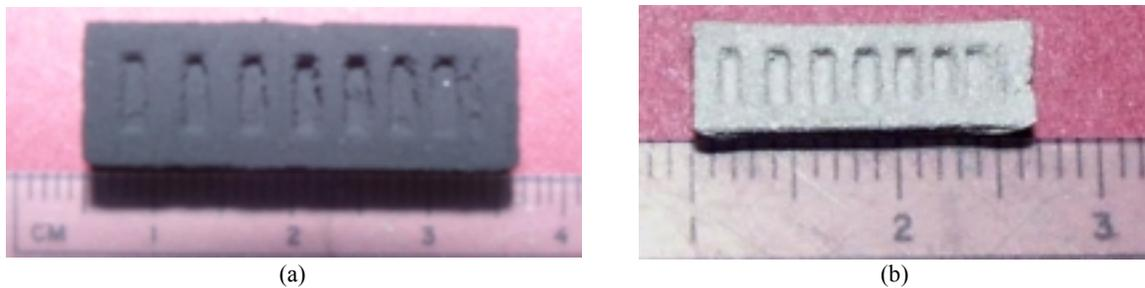
**Figure 6.** Thin wall test: (a) green part, (b) sintered and reduced part
