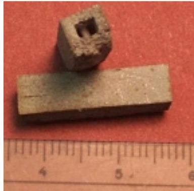
**Figure 8.** Sintered and reduced trussed channel test sample
