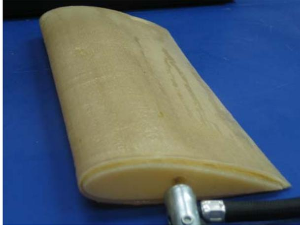
Figure 20. UAV wing inflated using air pump at  $1500\text{N/m}^2$  (gauge pressure).
