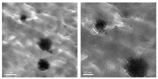
**Figure 1** TEM micrographs of polyamide 11 with 15% OP1311 (large dark micron-sized particles) and 5% Cloisite® 30B (hairline 1 nm thick platelets) polymer showing exfoliation of nanoclay in PA11 was achieved.
