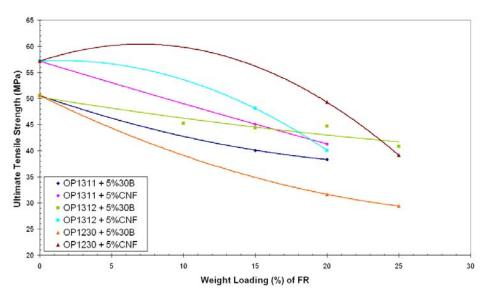
Figure 3 Ultimate tensile strength of PA11 FR nanocomposites with 5% nanoparticles.
