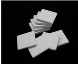
Fig. 4 Parts (10 x 10 mm) fabricated by the process of Ceramic Laser sintering
