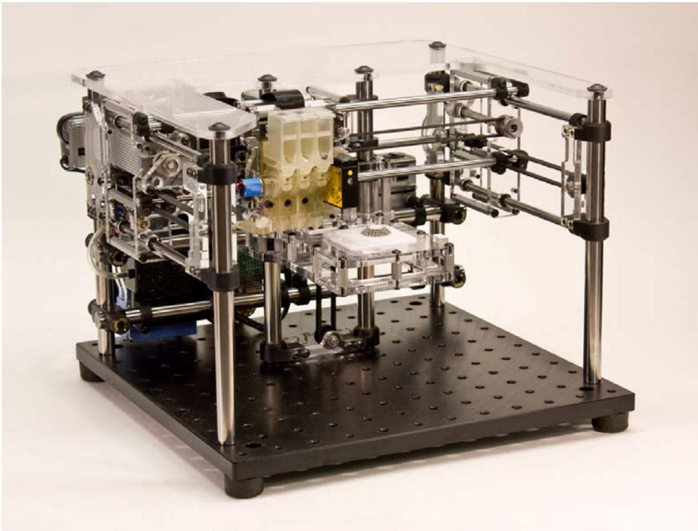
**Figure 2:** The VoxJet research platform was used to quickly and autonomously build multi-material structures made of hundreds of 1.5mm spherical voxels. The system also deposits binder to hold the structure together and includes error correction via closed loop deposition feedback.
