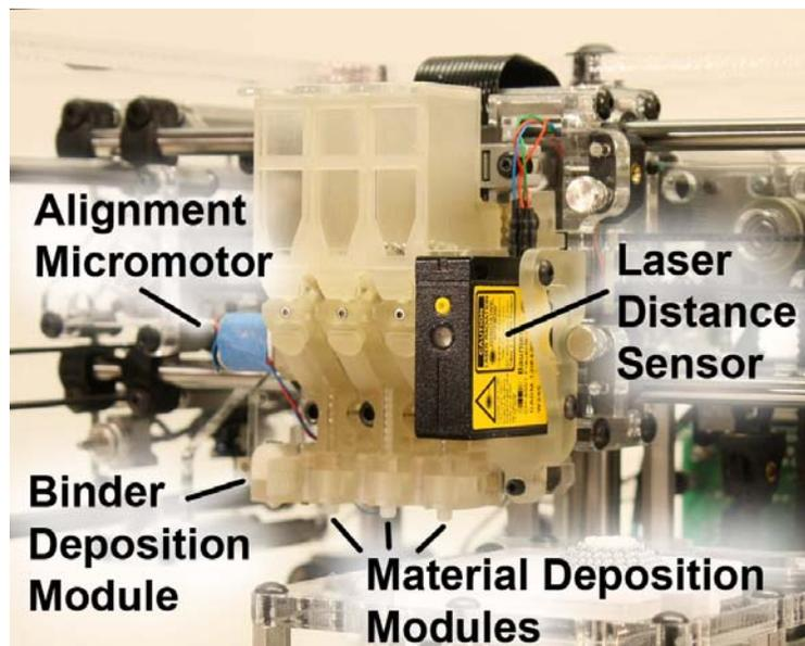
**Figure 4:** The deposition head consists of a binder depositing system, three separate material deposition modules, and a laser distance sensor. As the print head scans from right to left, binder is deposited appropriately, followed by spheres of any available material. The laser sensor verifies the placement of each sphere.
