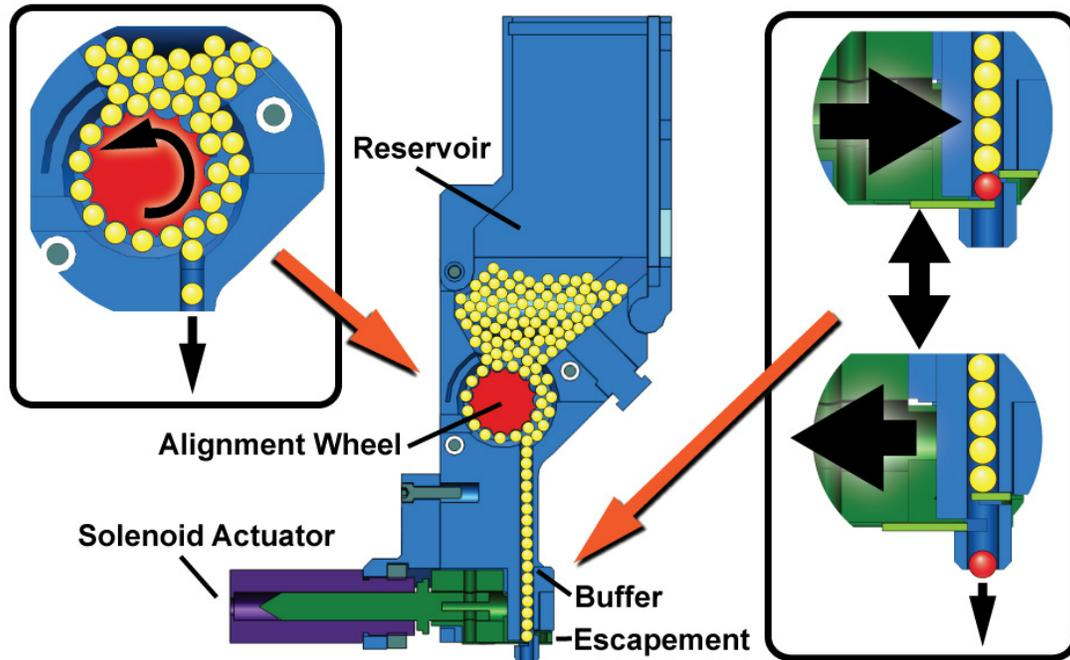
**Figure 3:** A cutaway diagram of the material deposition modules. Loose spheres are poured into the reservoir, which are aligned into a one-dimensional buffer by the continuously rotating alignment wheel. A solenoid actuated escapement mechanism deposits precisely one sphere with each cycle, and can reliably deposit up to ten spheres per second.
