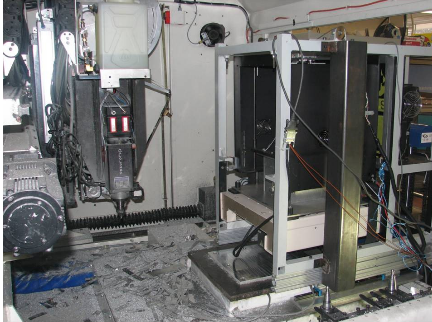
Figure 6: Flexible FDM machine slid into UC machine for deposition.
