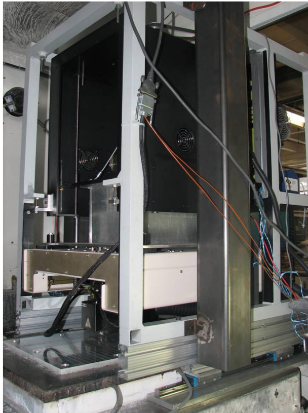
Figure 7: FDM machine positioned inside UC machine and ready for build.
