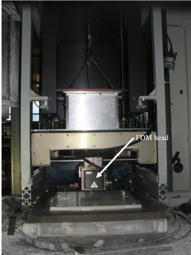
Figure 8: Front view of flexible FDM deposition system showing the FDM head.
