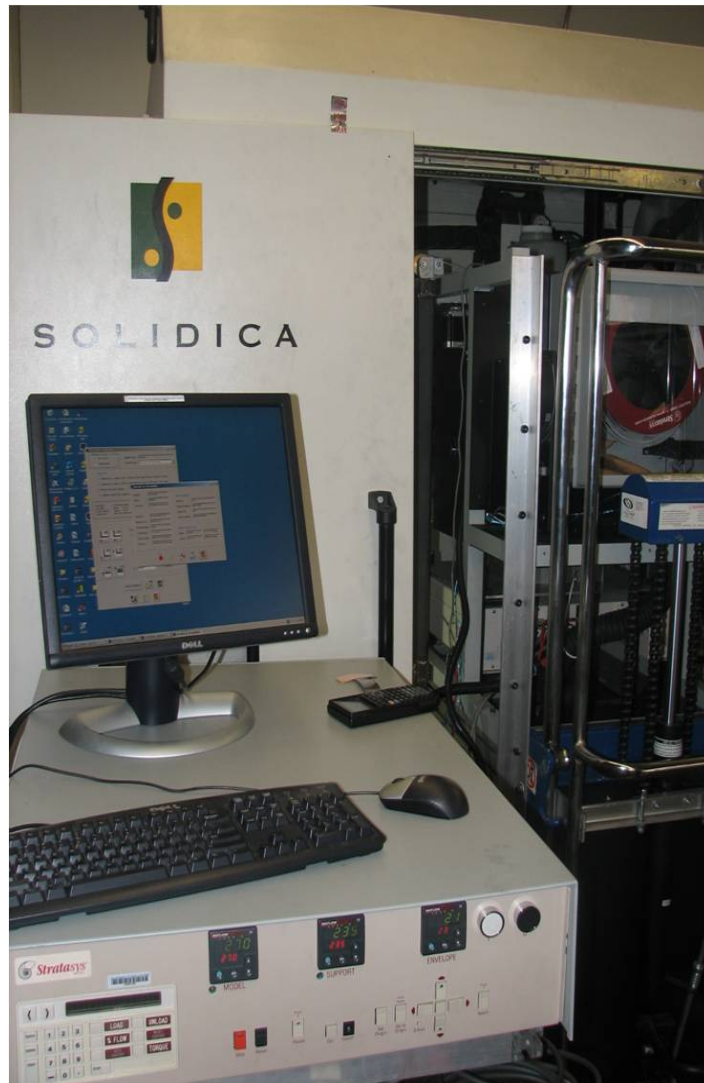
Figure 9: Combined Solidica UC machine with flexible FDM deposition system.
