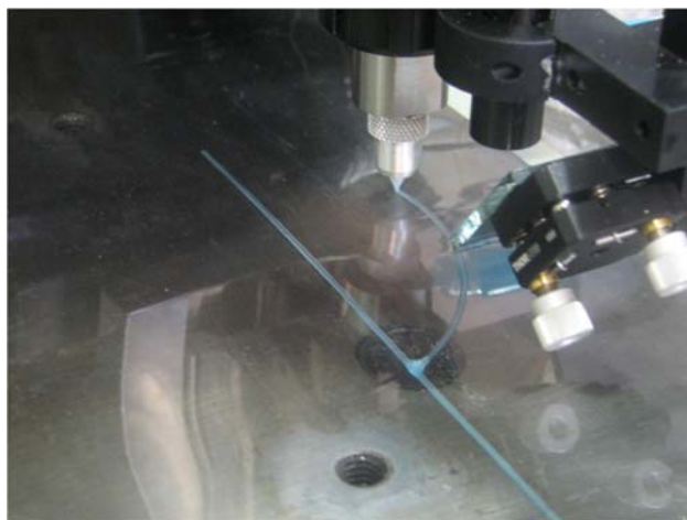
Figure 15: UC-DW integrated system dispensing onto a plastic substrate.
