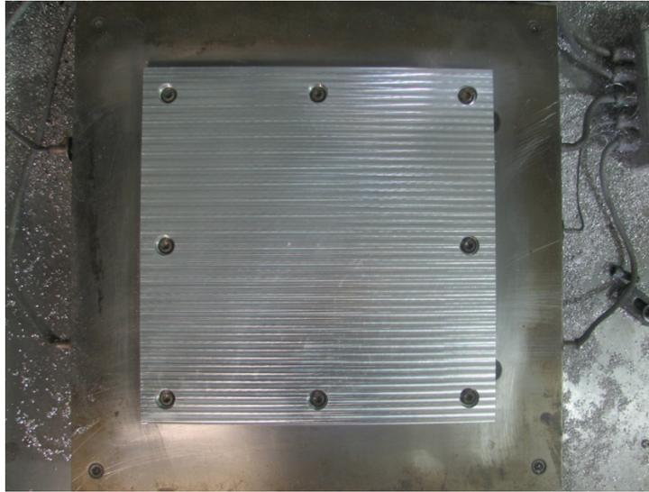
**Figure 4.** Geometry of the base plate used within the Solidica Formation™ machine and bolt locations just before deposition
