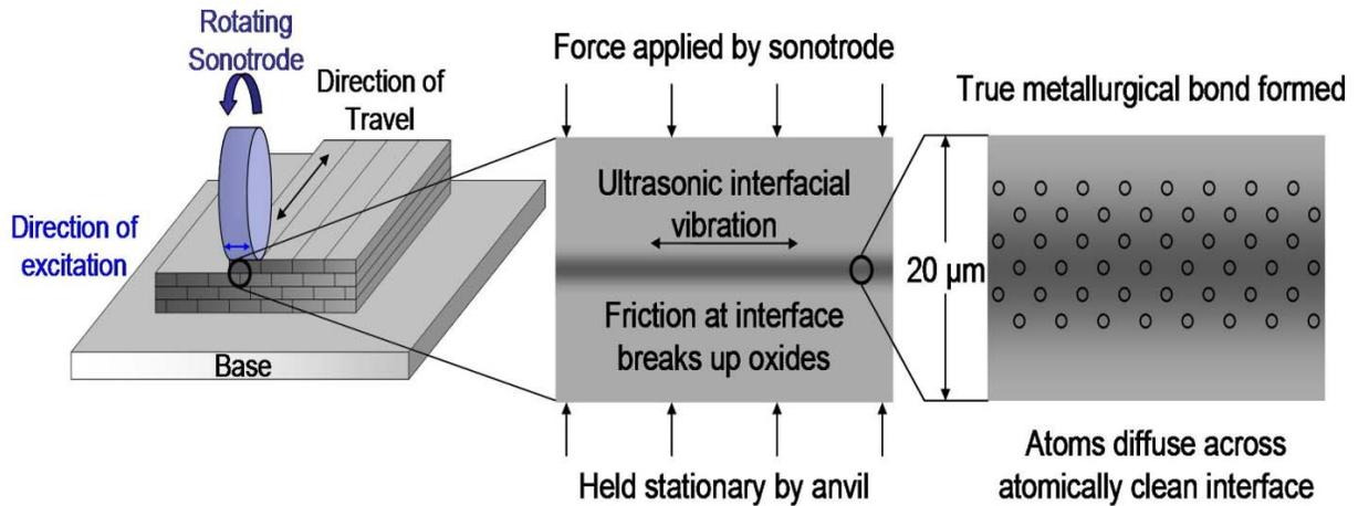
**Figure 1.** Schematic of the ultrasonic consolidation process
