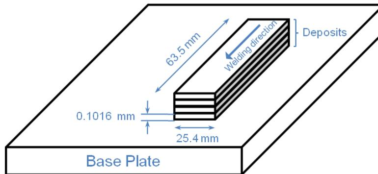
**Figure 7.** Schematics of the SS316L annealed UC sample
