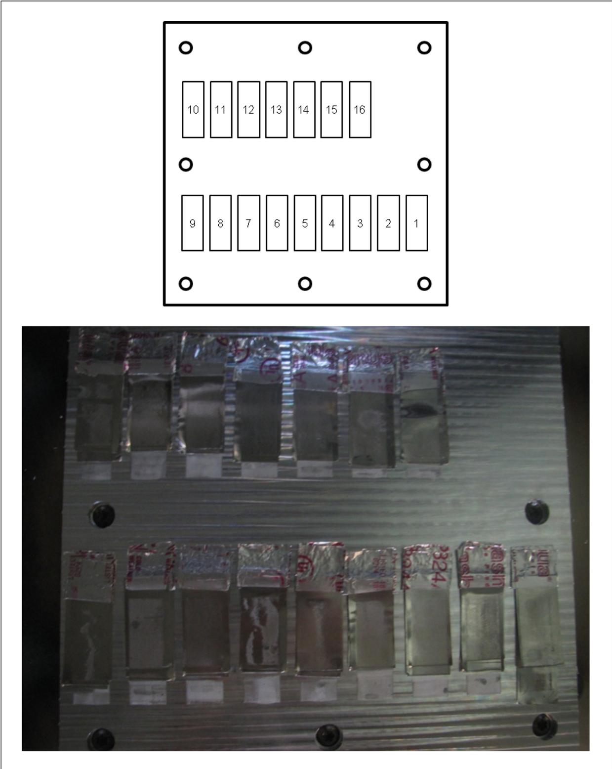
**Figure 8.** Actual experiment samples and layout of experiment runs on base plate
