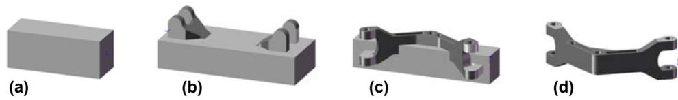
**Figure 1 – Multiple setups required (even in multi-axis milling) to create component via a subtractive process; (a) shows initial stock geometry and (b-d) show the results after iterative cutting operations until (d) the component fully emerges**
