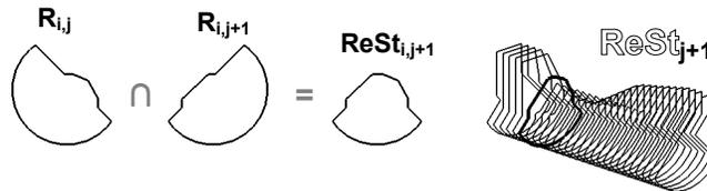
**Figure 11 – Each  $\text{ReSt}_{i,j}$  in  $\text{ReSt}_{j+1}$  is computed as the cumulative intersection of preceding single-cut effects  $\mathbb{R}_{i,j}$ , allowing independent computation of  $\mathbb{R}_{i,j}$**
