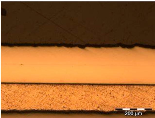
**Figure 8: Nickel/Stainless steel 316L welded on Al 6061-T6 substrate**
