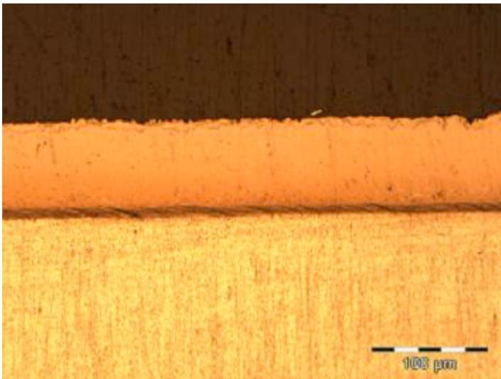
**a: Titanium/Al 3003 with elemental boron powder at the interface**
