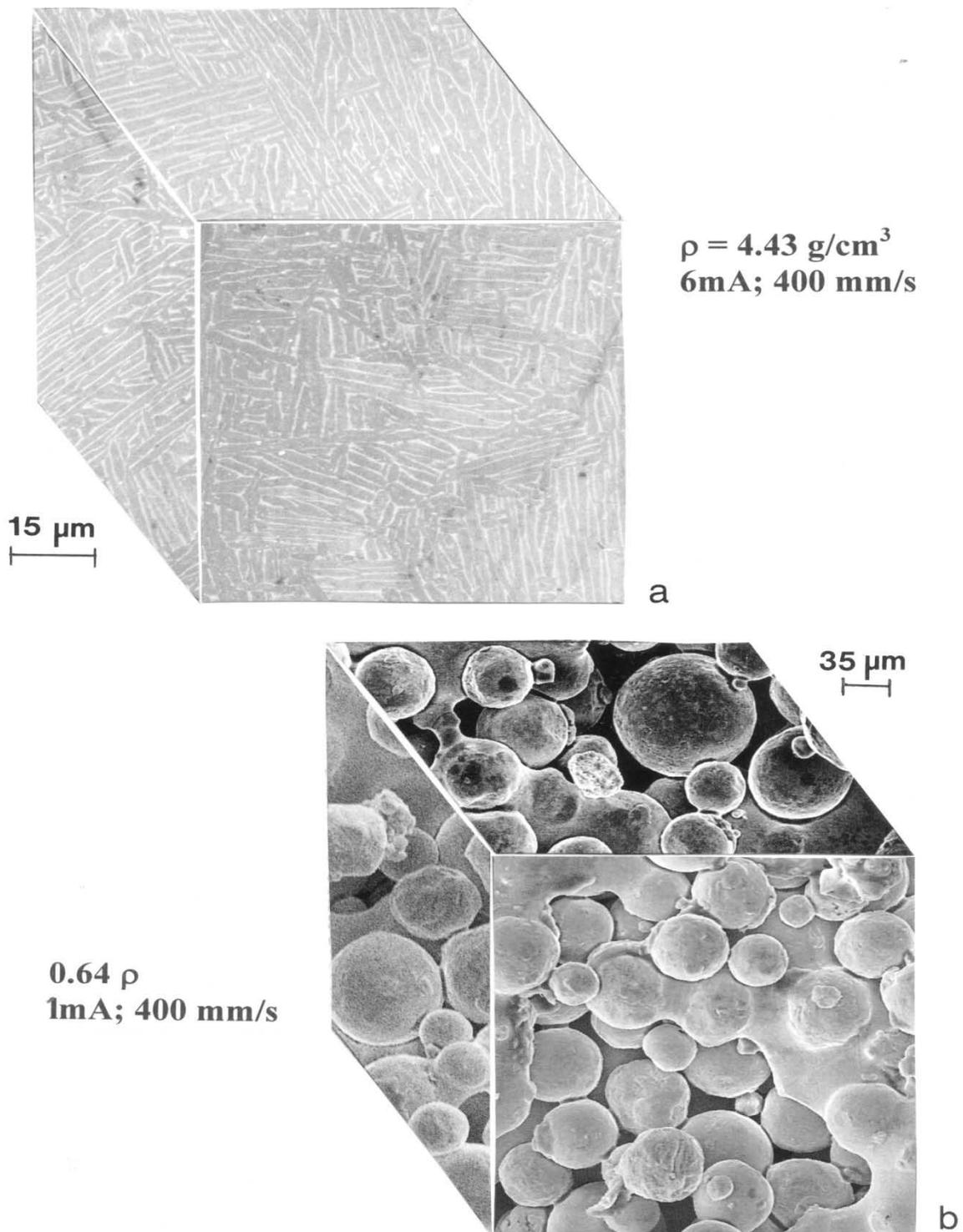
Figure 4. Ti-6Al-4V build comparisons. (a) Shows the optimized build parameters to produce fully dense monolith while (b) shows a reduction in melt-beam current. From Gaytan, et al., (2009).
