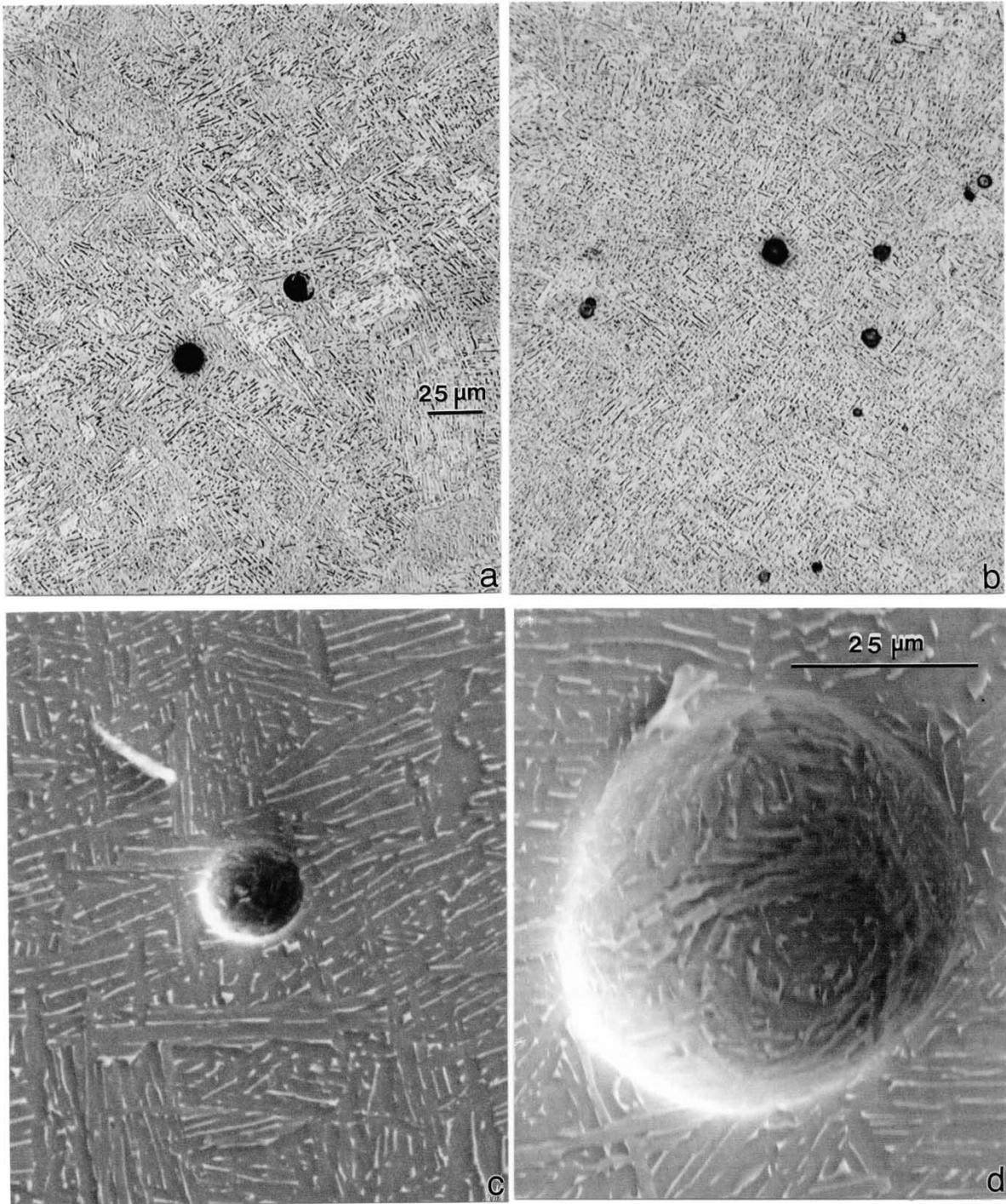
Figure 5. Examples of gas (void) bubbles in solid monoliths. (a) and (b) are optical metallograph images while (c) and (d) show SEM images.
