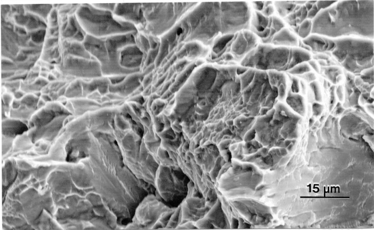
Figure 17. Low (a) and high (b) magnification SEM images of tensile specimen fracture surfaces. The specimen was machined from a triple (3) melt pass build of a 2 cm diameter, 8 cm long cylindrical specimen.
