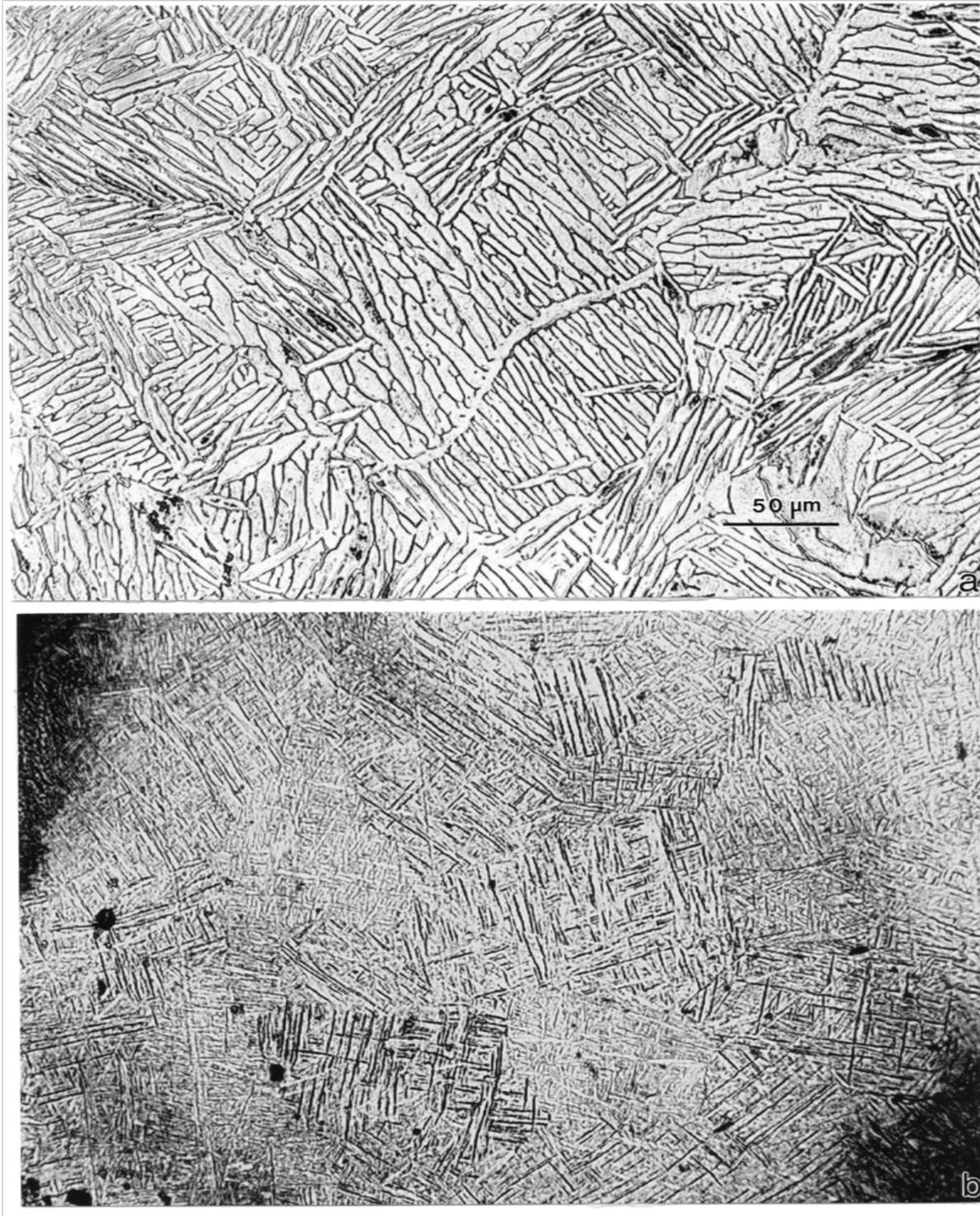
Figure 11. Comparison of residual microstructures for triple (3) melt pass fabrication of fully dense monolith in longitudinal plane (parallel to build direction) (a) with optimized single melt pass fabrication of 1.59 g/cm<sup>3</sup> dense, Materialise™ dode-thin element strut (as in Figure 9(f)) showing primarily  $\alpha'$  martensite platelets. From Murr, et al. (2009c).
