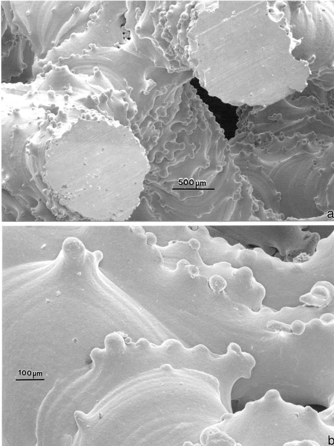
Figure 13. (a) SEM views of cut and polished cellular bridges in the center foam ( $0.68 \text{ g/cm}^3$ ) in Figure 12(a). (b) Magnified view of foam cells showing layering and edge-sintered powder particles.
