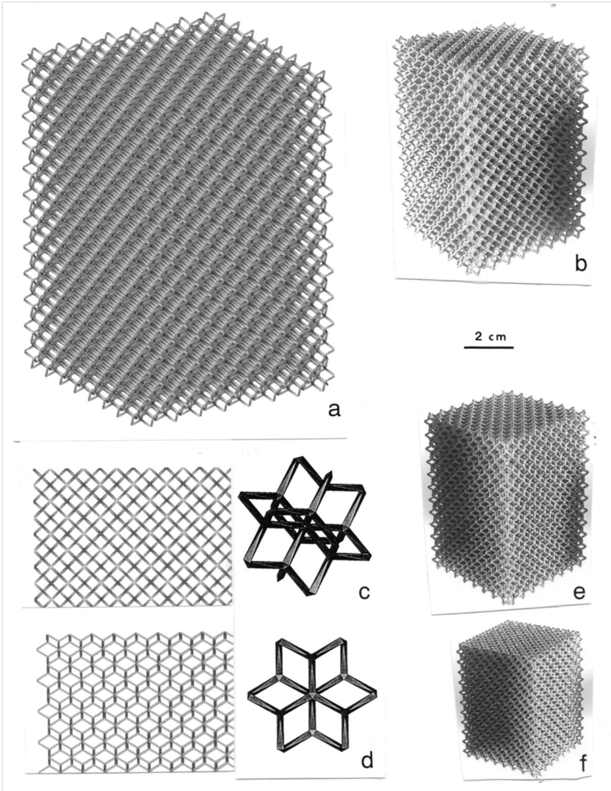
Figure 9. Software model views and EBM fabricated prototypes utilizing the Materialise™ dode-thin software element. (a) shows the software model while (b) shows the corresponding build. (c) and (d) show dode-thin element orientations which correspond to hexahedral and octahedral geometries occurring in the “faces” and diagonals (at 45°) in the structures. (e) and (f) show smaller mesh builds. From Murr, et al. (2009c).
