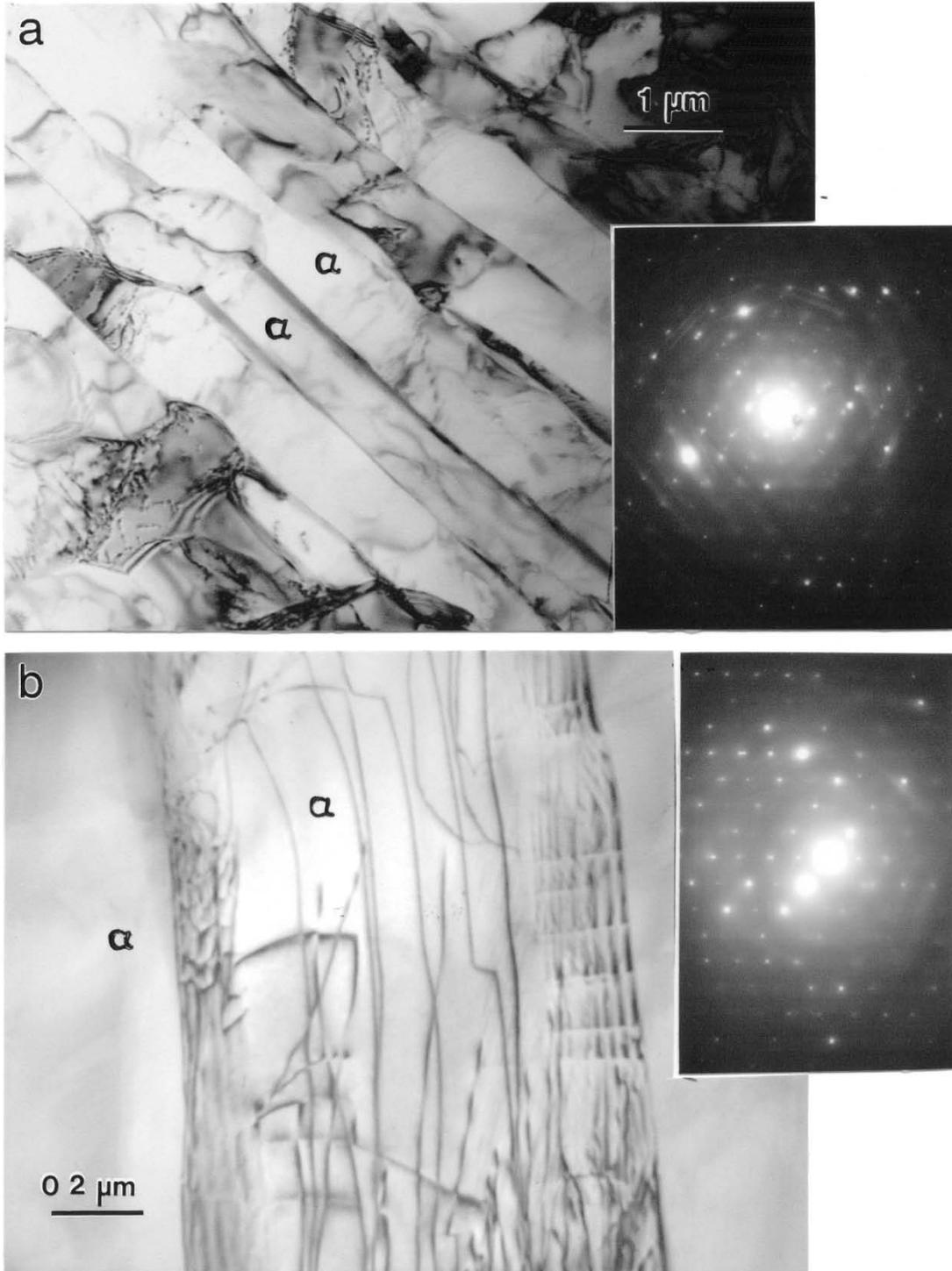
Figure 16. TEM bright-field image comparisons for (a) 0.91 mm thick “window” section corresponding to Figure 2(b), and (b) 0.64 mm thick “window” section corresponding to Figure 2(b). The selected-area electron diffraction pattern inserts show the same crystallographic orientation for (a) and (b).
