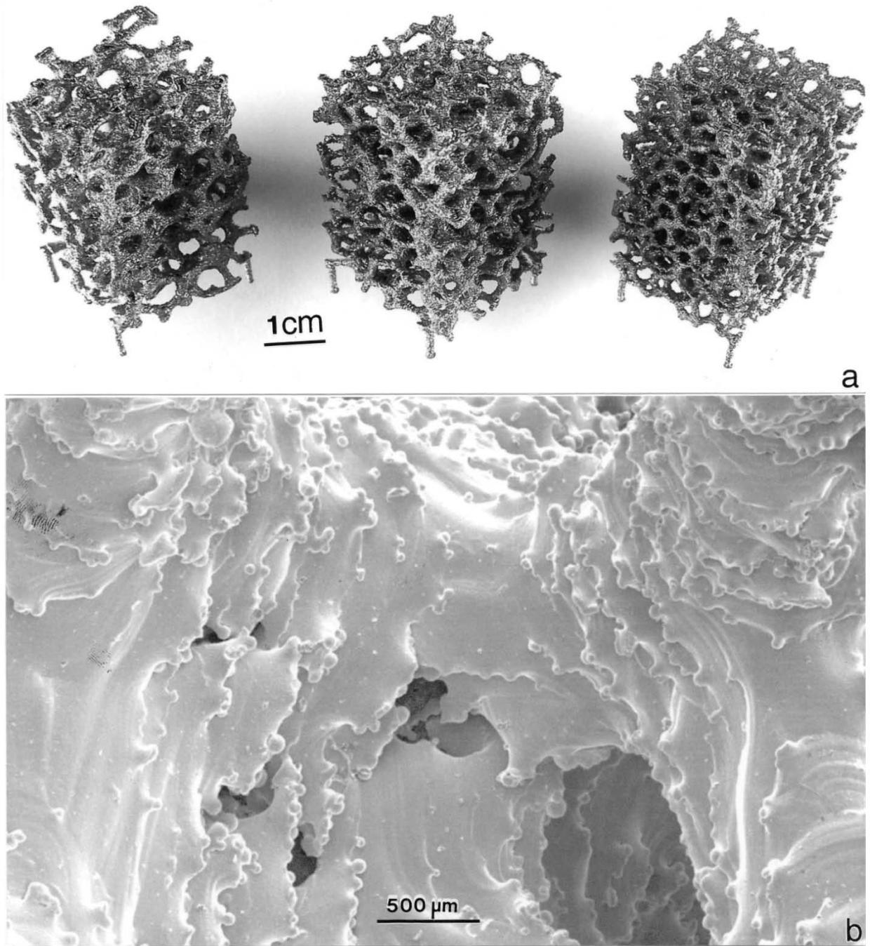
Figure 12. Three Ti-6Al-4V foam prototypes (a) and an SEM view of the center foam prototype (b). The foam prototypes in (a) correspond to (from left) 0.58, 0.68, and 0.83 g/cm<sup>3</sup> densities, respectively.
