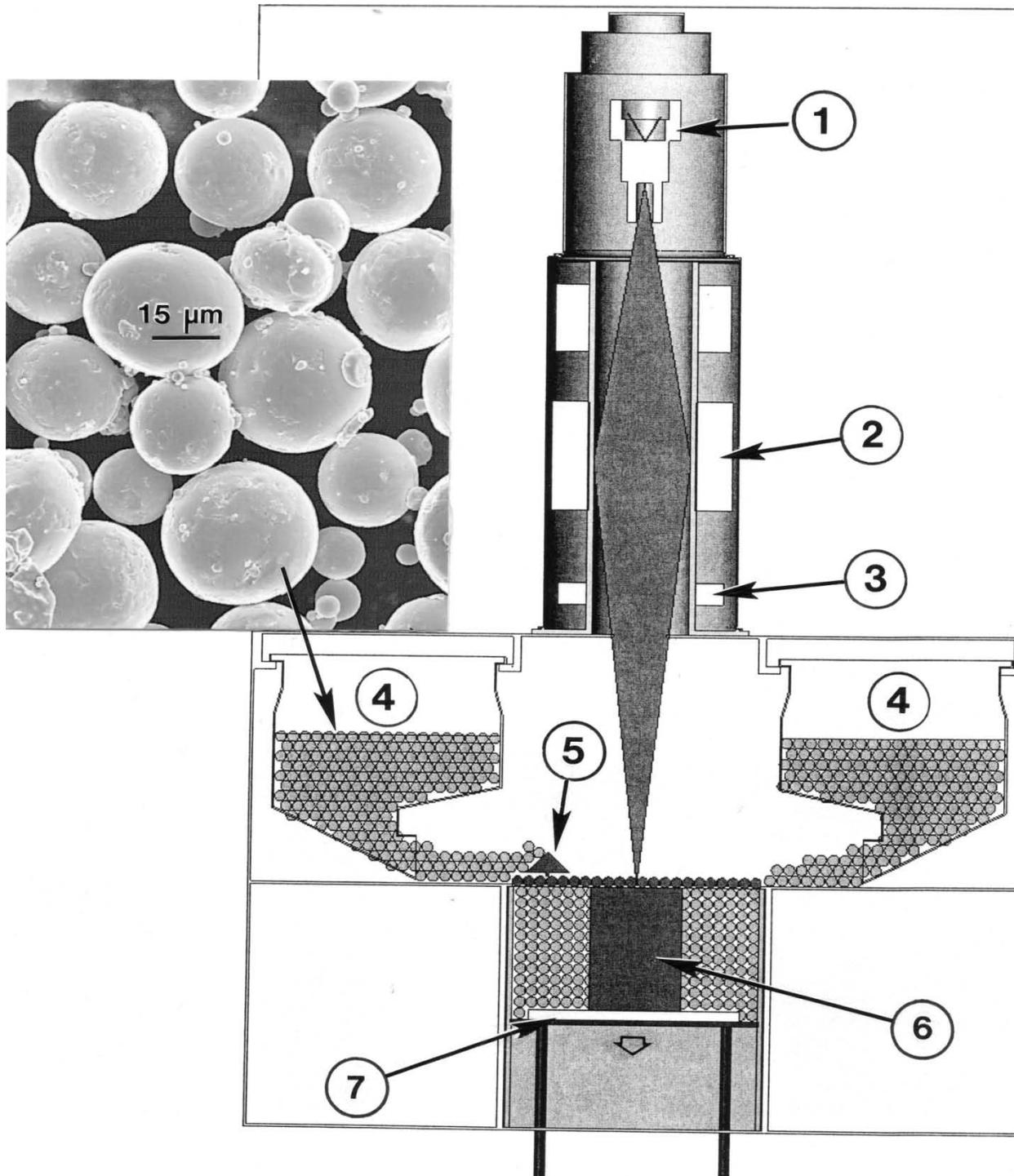
Figure 1. EBM schematic and SEM view of precursor powder (insert). Numbers denote the system components: (1) Electron gun, (2) Beam focus lens, (3) Beam deflection coils, (4) Powder cassettes, (5) Powder layer rake, (6) Build product, (7) Build table. From Gaytan, et al. (2009).
