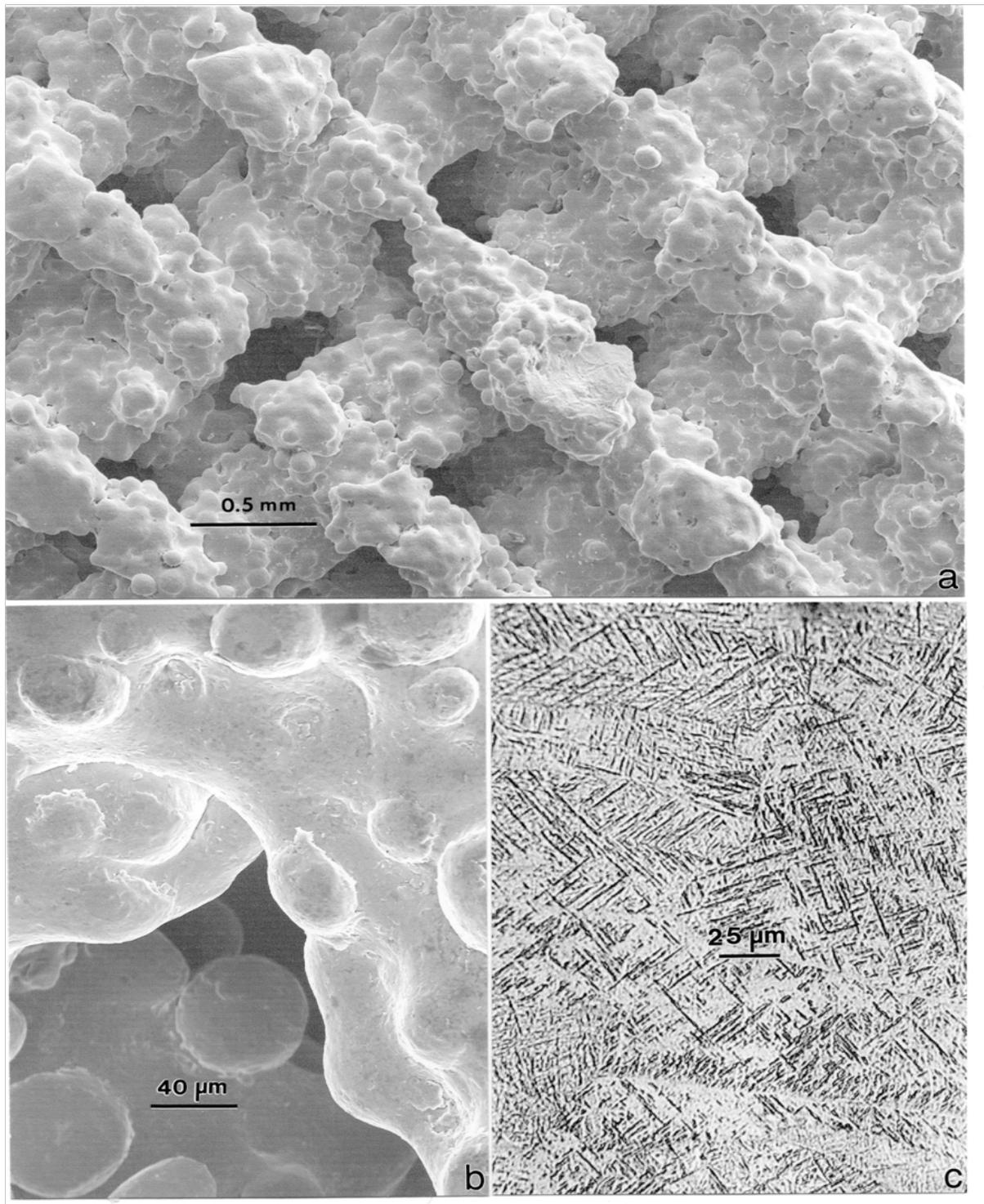
Figure 10. SEM and optical metallographic images of the dodecagonal mesh component in Figure 9(f). (a) Square (hexahedral) mesh geometry in SEM. (b) Magnified view of (a). (c) Optical microscopy image showing primarily  $\alpha'$  martensite platelets intermixed with some  $\alpha$ -phase on polished and etched connecting strut in (a). From Gaytan, et al. (2009).
