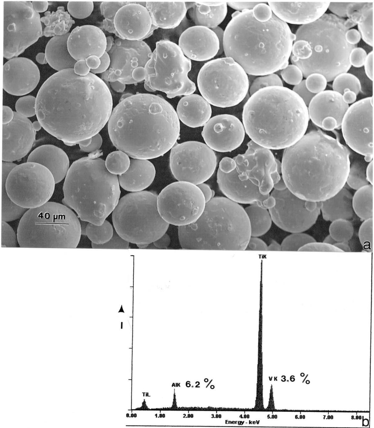
Figure 8. EDS analysis of individual powder particles after 10 cycles of mixed reuse (breakaway powder added to recycled powder). (a) SEM image of Ti-6Al-4V powder for comparison with the precursor powder insert in Figure 1. (b) EDS analysis of a single, random particle in (a). From Gaytan, et al. (2009).
