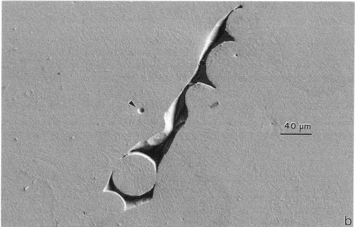
Figure 3. Examples of build defects. (a) Unmelted and consolidated zone. (b) is similar to (a) with gas void (exposed bubble) at arrow. From Gaytan, et al. (2009).
