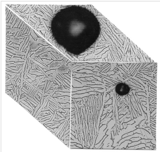
Figure 7. Series of 3D reconstructions of optical metallograph views for solid monoliths built with optimum melt scan parameters, but with (a) one melt scan, (b) two melt scans, (c) three melt scans. The bubble density is exaggerated in each case. Note variation in  $\alpha$ -phase grain structure dimensions from (a) to (c). Magnifications the same as shown in (a).
