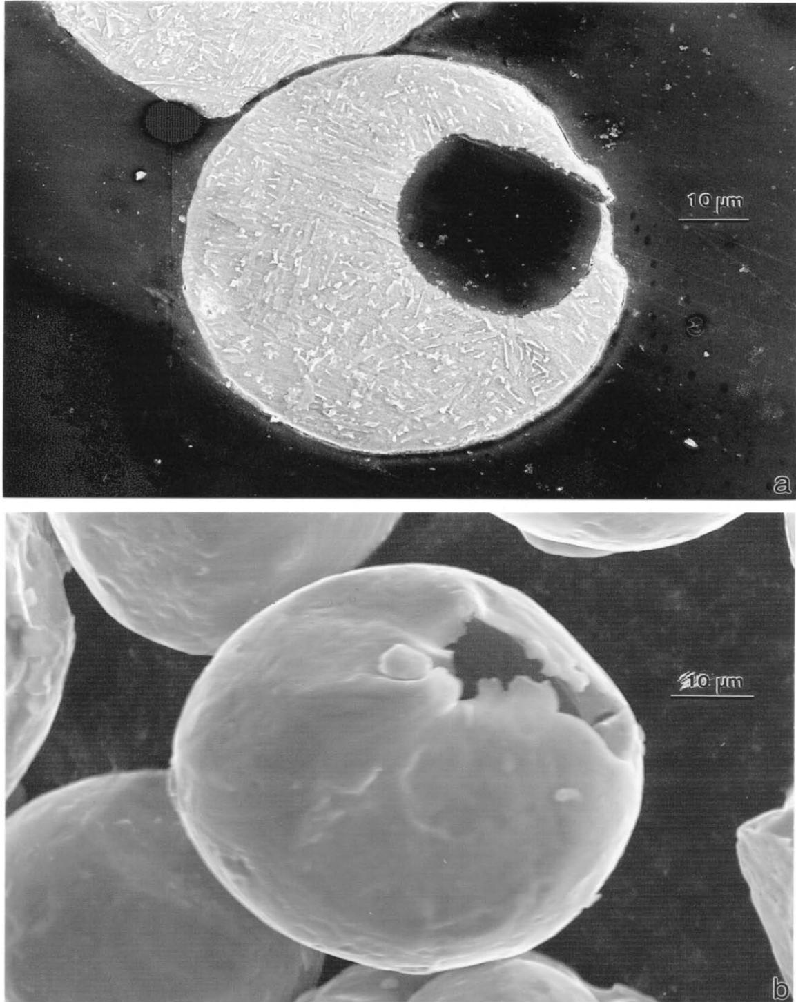
Figure 6. Gas bubbles in Ti-6Al-4V powders (typical for precursor/starting powder and recycled powder). (a) SEM metallographic view of mounted, ground, polished, and etched powder particle showing interior void. (b) SEM view of gas bubble breaking the powder particle surface. From Gaytan, et al. (2009).
