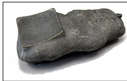
Fig.8. SLsed A6 tool steel part pre-sintered from a relative density of 0.46 to 0.52 by heating to 1100°C for 3hrs and then infiltrated at 1310°C. As the infiltration temperature for given brown density lies in Region II, melting of tool steel along with cast iron is observed, distorting the final part.
