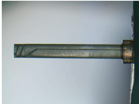
Fig. 11 Successfully built sleeve using multiple exposure
