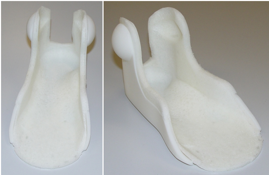
Figure 7: Mating of custom molded variable-thickness foam insert to stiff additively-manufactured polyamide (nylon) outer shell. The fit is nearly perfect due the accuracy of the fabrication processes involved.
