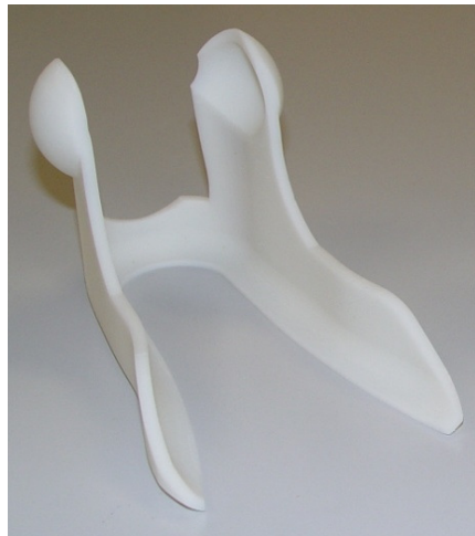
Figure 4: Hard shell of one custom pedorthosis produced in the Milwaukee School of Engineering's Rapid Prototyping Center® on a SLS machine.
