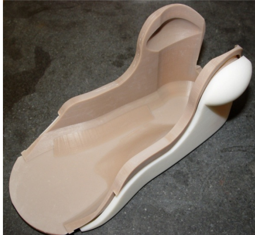
Figure 5: Light-brown SLA soft-layer pattern, set inside white SLA hard-shell pattern.
