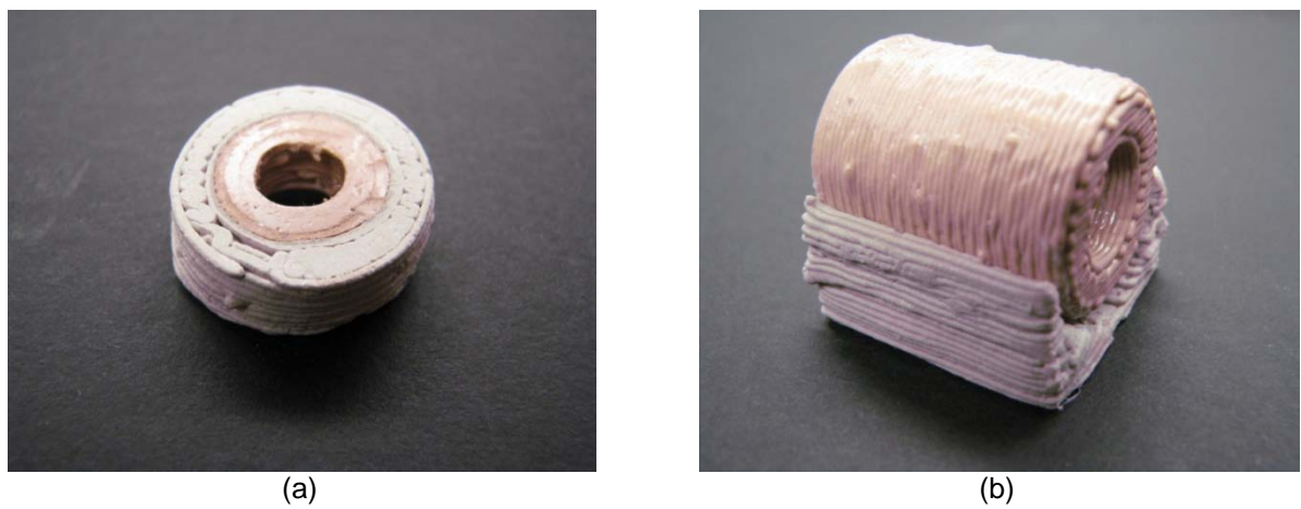
Figure 6: FabEpoxy pipes can be embedded into cement structure by simultaneously printing the materials (a) or by mechanical insertion after successful printing (b).
