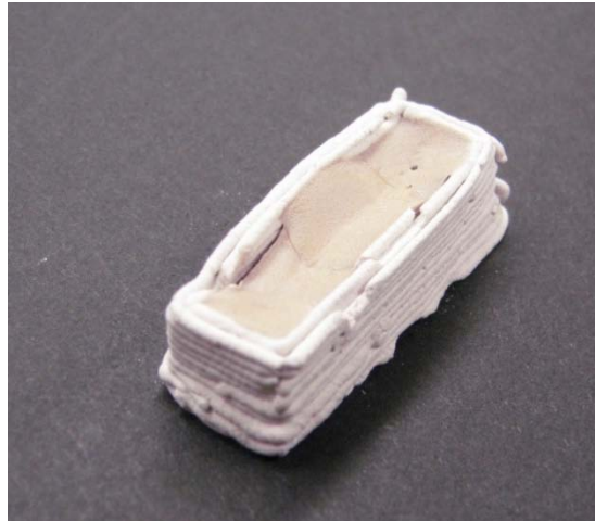
Figure 7: A section of printed electrically conductive silicone embedded in a printed cement structure.
