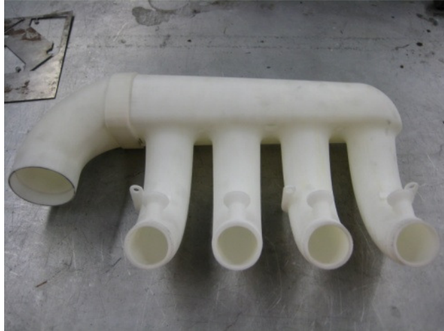
Figure 6. Final assembly of the intake manifold.
