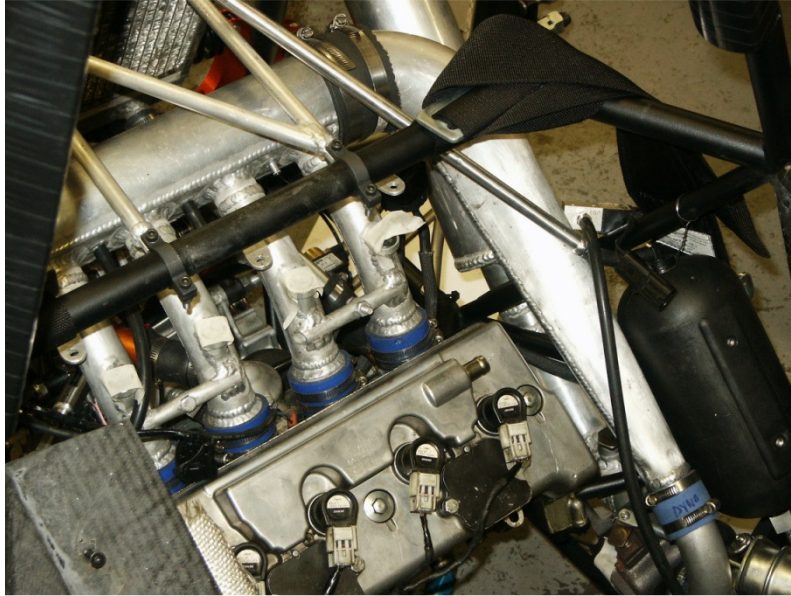
Figure 2. Intake manifold composed of welded aluminum pieces.
