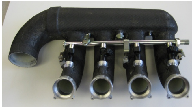
Figure 7. Completed intake system, following the composite layup process and final assembly of sensors and mounts.
