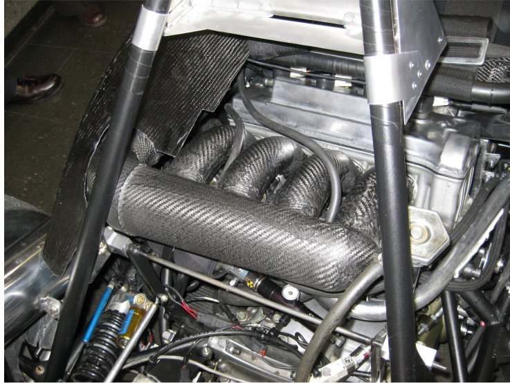
Figure 8. The intake system as mounted onto the 2009 Virginia Tech Formula SAE car
