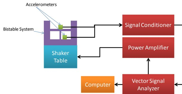
**Figure 14: Schematic of dynamic buckled beam test**
