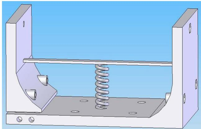
Figure 5: SolidWorks model of a buckled beam system
