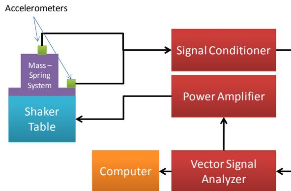
**Figure 8: Schematic for dynamic shear modulus test**
