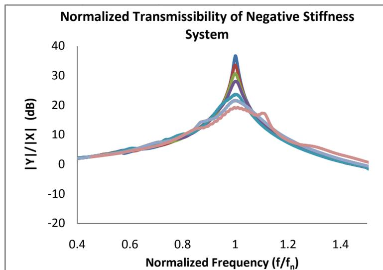
**Figure 16: Frequency normalized response of system during buckling**
