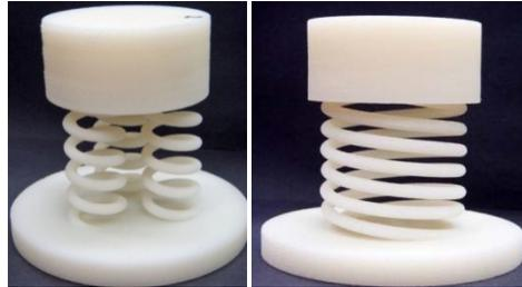
**Figure 7: Two different mass-spring systems used for dynamic testing. The system on the left contains three springs and the one on the right has two springs in a “double helix” configuration for stability of the mass**
