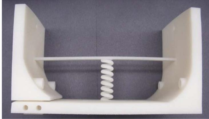
**Figure 13: The buckled beam system made of Nylon 11**
