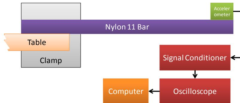
**Figure 9: Schematic for Young's modulus dynamic test**
