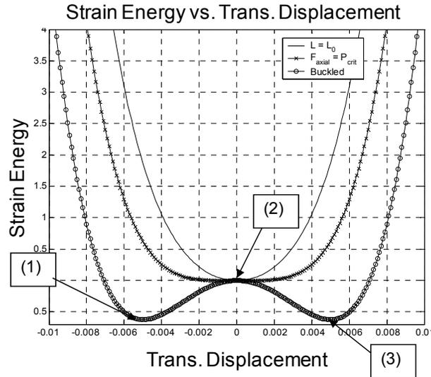
**Figure 3: Plot of strain energy vs. transient displacement. Points (1), (2) and (3) match those in Figure 2 as well as the legend for the unbuckled, critically buckled and completely buckled states. Image from Haberman, 2007.**
