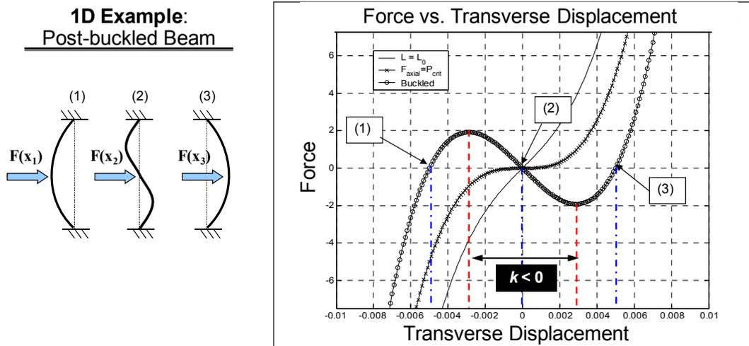
**Figure 2: Plot of the force vs. displacement of the center of a beam in the transverse direction. The line with x's represents a beam that is critically buckled, while the line with circles represents a beam that is past the critical buckling range and is displaying negative stiffness in the region marked  $k < 0$ . The solid line shows the response for an unbuckled beam. The stages of snap-through in the buckled beam on the left are marked on the graph. Image from Haberman, 2007.**
