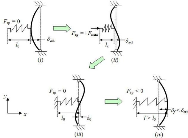
**Figure 1: Stages of snap-through movement of a buckled beam. (i) The beam is in an initial stable buckled state. (ii) A force is applied to the spring and sends the beam to the meta-stable state. (iii) The spring is constrained, and a slight change in displacement sends the beam to (iv) the second stable buckled state. Image from Haberman, 2007.**
