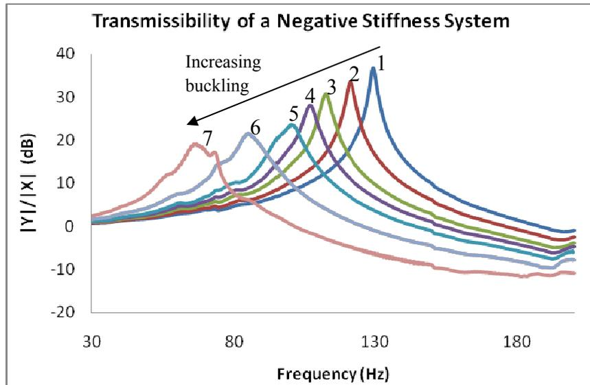
**Figure 15: Response of system during increased buckling. The curves are numbered for future reference.**
