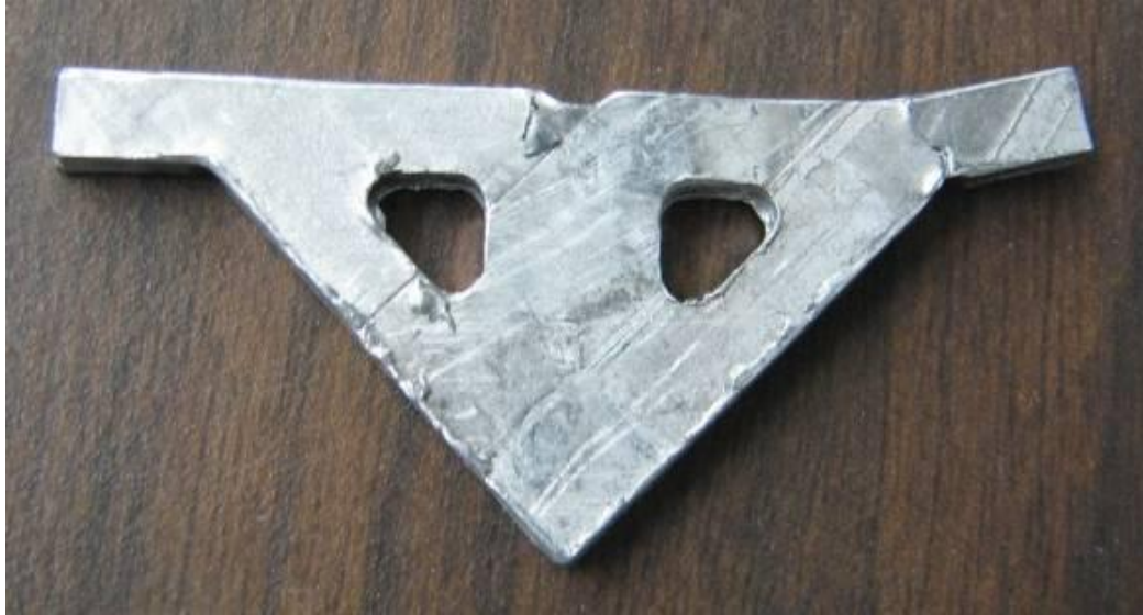
Figure 9: Failure feature of a structure designed based on maximum stiffness criterion
