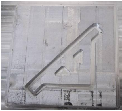
(f): The structure profile machined using UC integrated CNC milling
