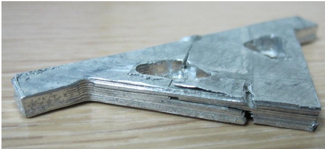
Figure 12: Fracture at both the edge-to-edge foil joint of the matrix material and the edge-to-edge joint of the reinforcing foils on a MetPreg ® reinforced tension member.
