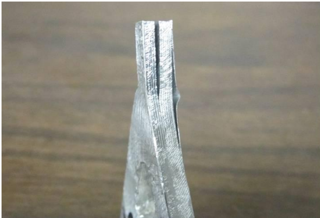
Figure 10: Delamination at the flange for some of the structures designed based on the maximum stiffness criterion
