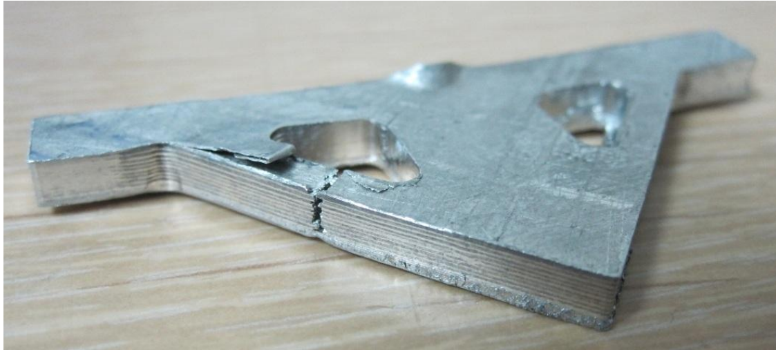
Figure 11: Fracture at the edge-to-edge foil joint of the matrix material on a MetPreg ® reinforced tension member.
