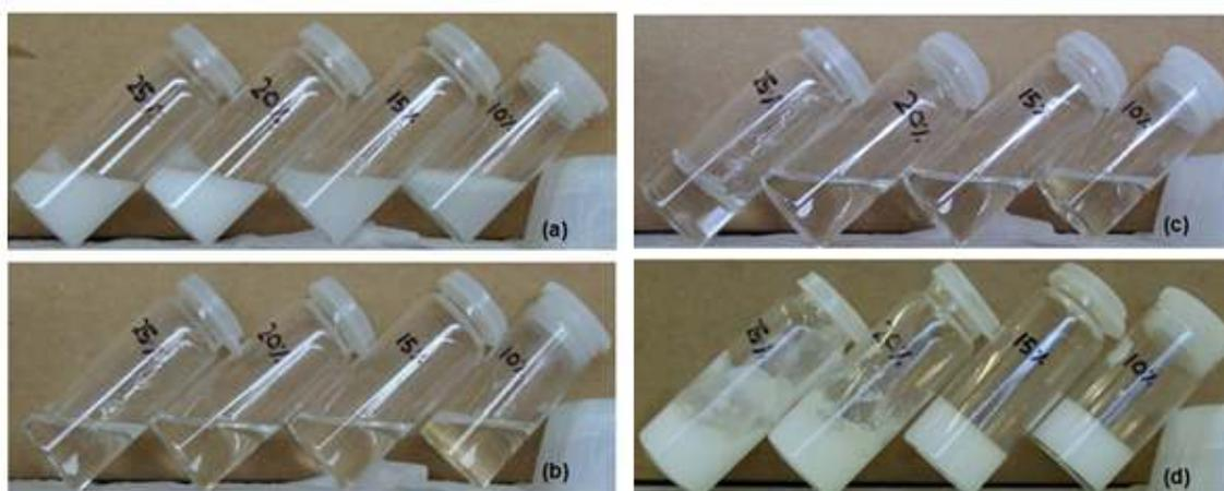
**Figure 1.** Pluronic F-127 in Ethylene Glycol samples at: (a) 20°C (b) 150°C (c) 50°C, during cooling (d) 25°C, cooled back
