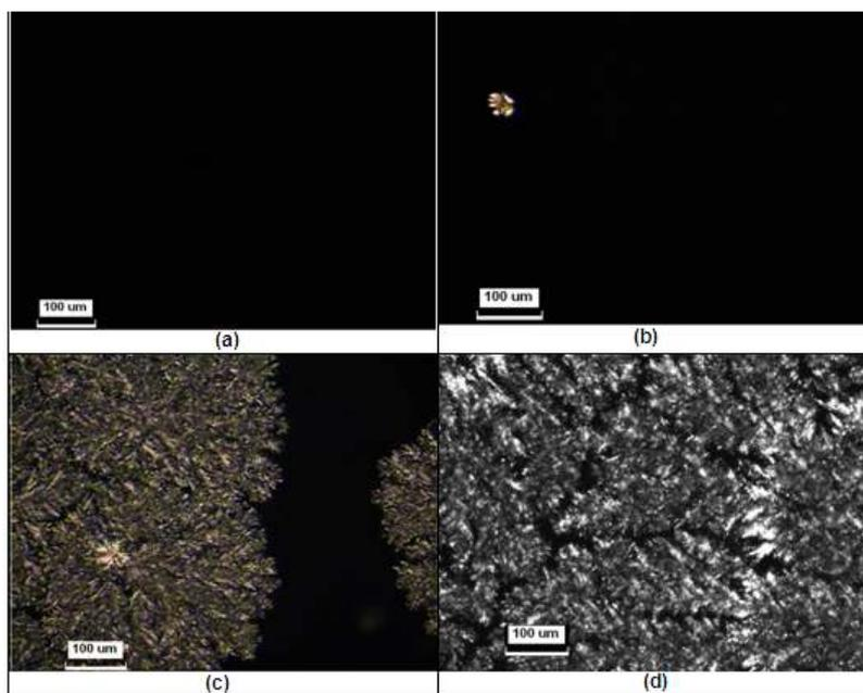
**Figure 4.** Micrographs of 25% Pluronic in Ethylene Glycol, cooled to: (a) 40°C (b) 28°C (c) 25°C (d) 25°C, after approximately 20 minutes
