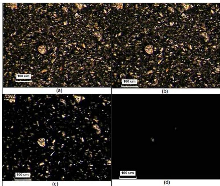
**Figure 3.** Micrographs of 25% Pluronic in Ethylene Glycol, heated at: (a) 25°C (b) 40°C (c) 42°C, dissolution increased (d) 44°C, completely dissolved
