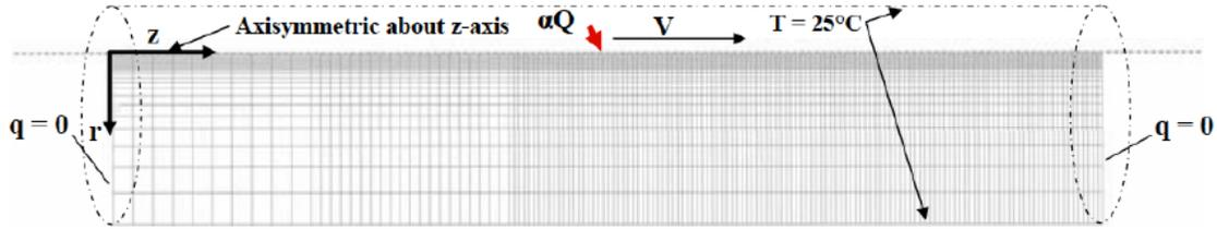
Figure 7: Representative 2-D Axisymmetric Finite Element Mesh for Transient Analysis
