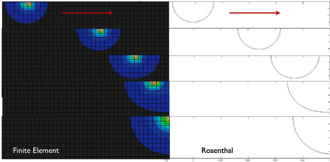
Figure 8: Melt Pool Contours Approaching Free-Edge
