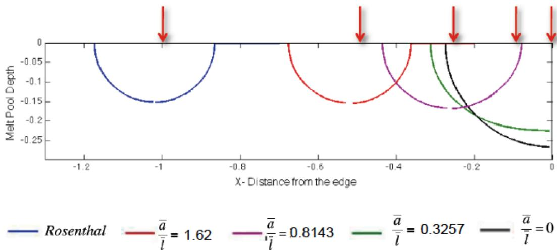
Figure 3: Small-Scale Process Melt Pool Geometry,  $\bar{T}_m = 2.88$
