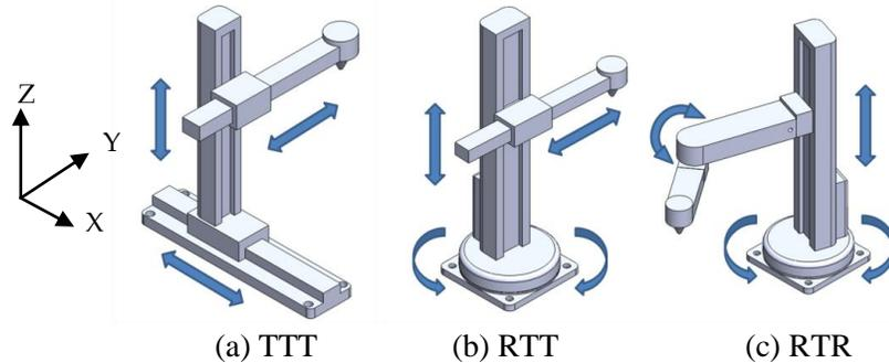
Fig. 4. Manipulation modules with common 3-DOF topologies
