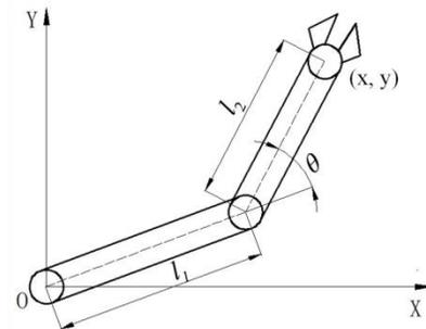
Fig. 6. A typical 2-DOF planar structure
