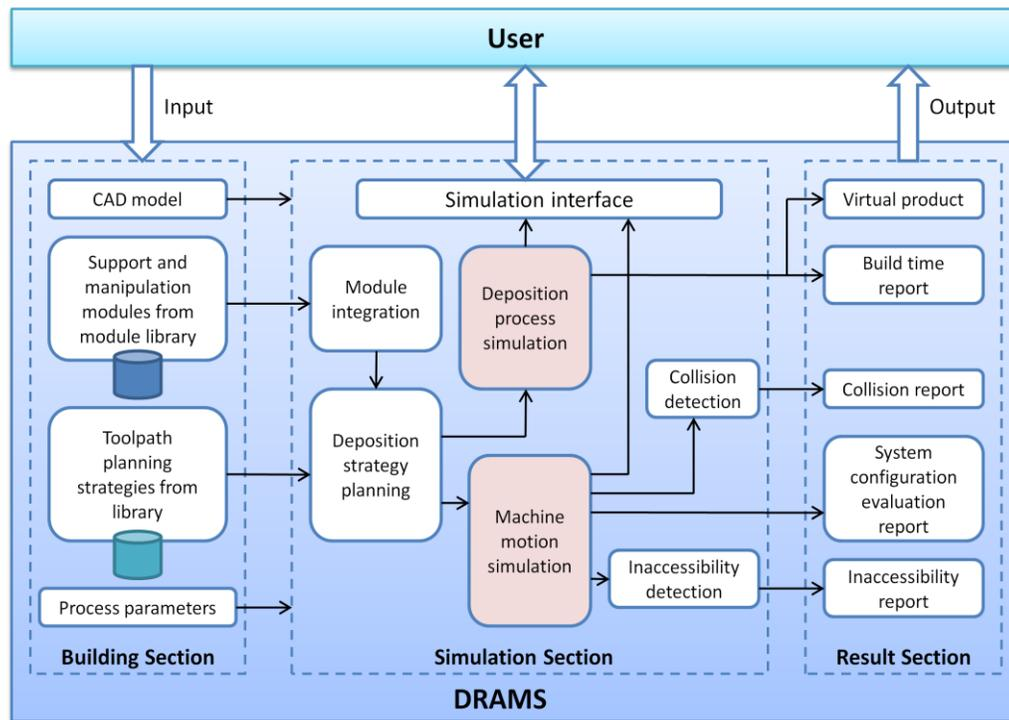
Fig. 1. Main elements and flow of the DRAMS
