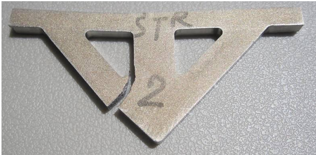
(a): Failure at a tension member on an STR10 structure
