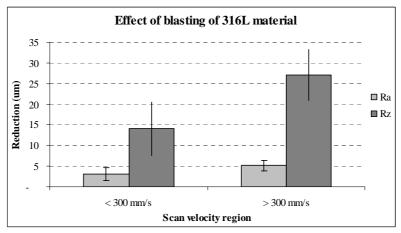
Figure 4: Effect of a blasting operation on Ra for scan velocities of < and > 300 mm/s
