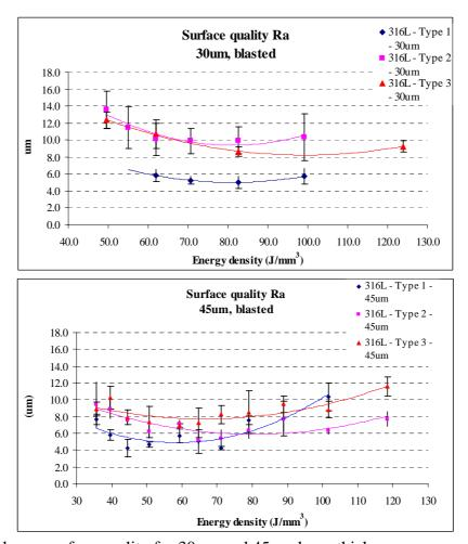
Figure 3: Blasted scan surface quality for 30µm and 45µm layer thicknesses
