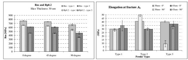
Figure 6: Ultmate tensile strength R<sub>m</sub> and yield strength at 0.2% offset R<sub>p0.2</sub> for 0°, 45° and 90° orientations (left) and elongation at fracture A<sub>t</sub> (right) for powder type 1 and 3.
