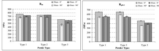
Figure 5: Ultmate tensile strength R<sub>m</sub> and yield strength at 0.2% offset R<sub>p0.2</sub> for powder types 1, 2 and 3 for 30 $\mu$ m- and 45 $\mu$ m-layers and for the two specimen orientations  $0^{\circ}$  and  $90^{\circ}$
