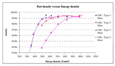
Figure 2: Part density versus Energy density for 30µm and 45µm layers
