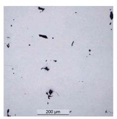
Figure 7: Pore sizes of test cubes for powder type 1 (left) and type 3 (right) for  $30\mu m$  layers in  $0^\circ$  orientation
