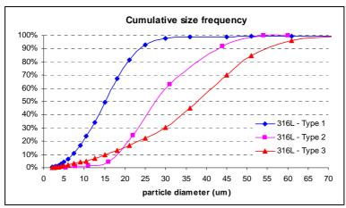
Figure 1: Cumulative size frequencies of powder type 1, 2 and 3
