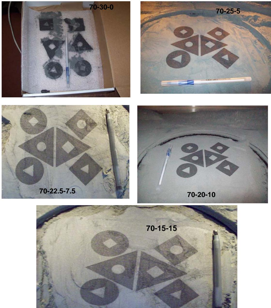
Figure 4: Single layer scan parts with different binder composition
