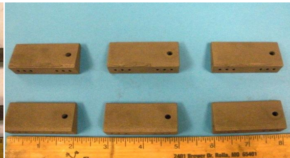
Figure 4 Successful green injector parts
