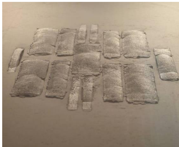
Figure 2 Warping of the 2 nd layers after laser scanning
