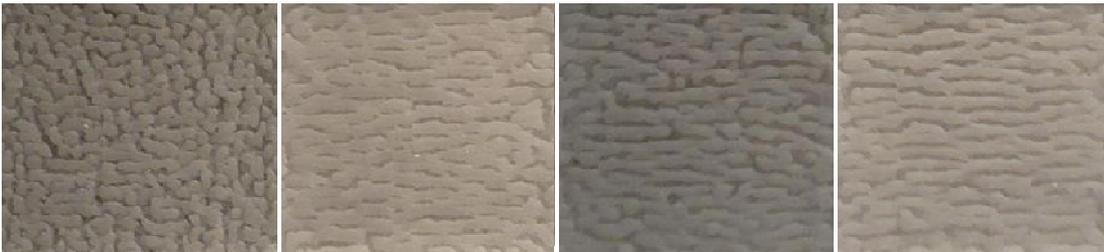
(c) Effect of Laser power (L-R: 15, 20, 22 and 25 W) at Scan speed = 50.8 mm/s and Scan spacing = 0.076 mm
