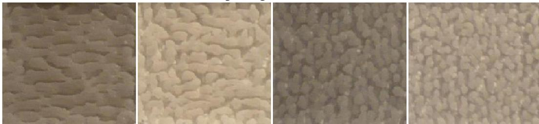
(b) Effect of Scan spacing (L-R: 0.076, 0.101, 0.127 and 0.152 mm) at Laser power = 25W and Scan speed = 50.8 mm/s
