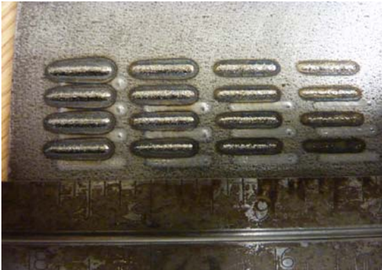
Figure 9: Experimental deposits of tribaloy - 400
