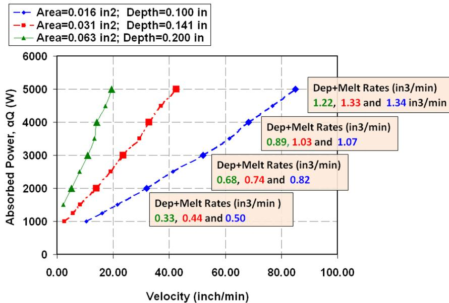
**Figure 1.** Analytical predictions for power and velocity combinations yielding constant cross sectional areas
