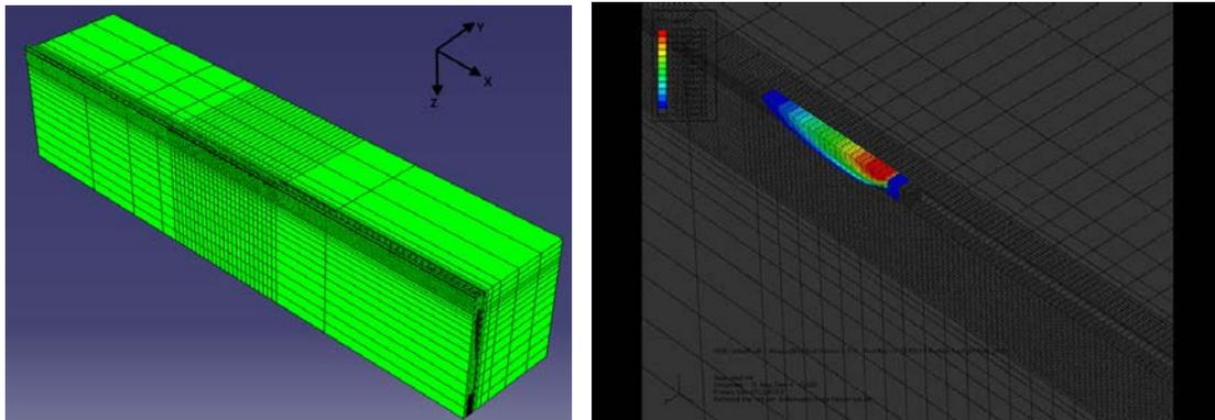
(a) Added material and constant bead 3-D model geometry and mesh
