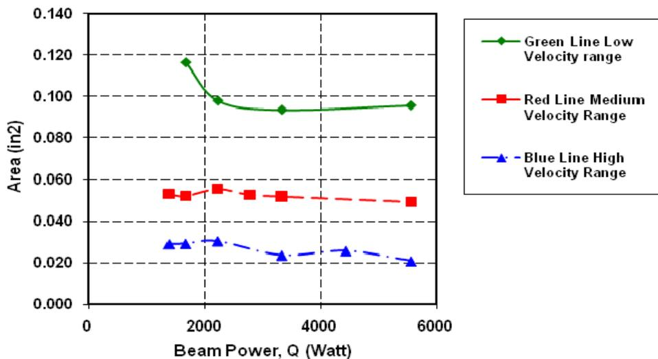
**Figure 5.** Experimental results presenting total (deposited+melted) cross section areas with changing power. Velocities were selected according to fitted Rosenthal calculations to obtain a constant area.
