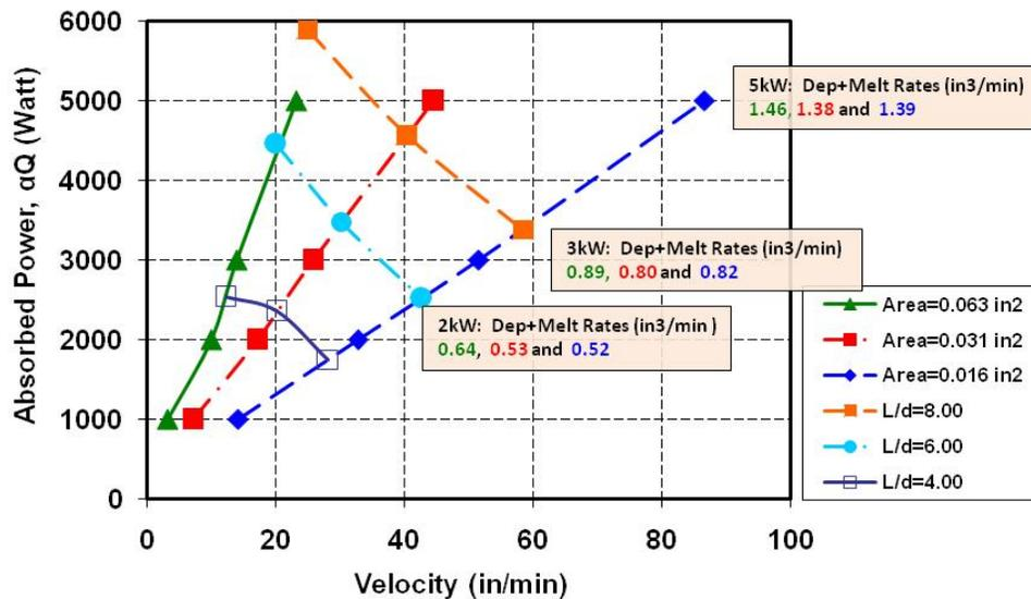
**Figure 3.** Lines of constant melted cross sectional areas and L/d ratios as determined by added material finite element simulations
