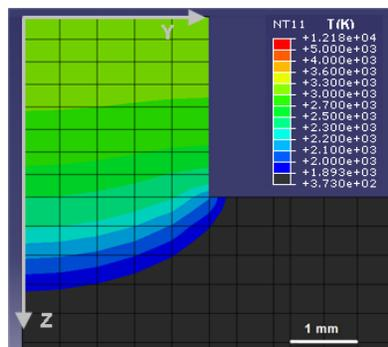
(c) Maximum cross section area of the melt pool (image is a cross sectional cut view of the geometry shown in (a) and (b))
