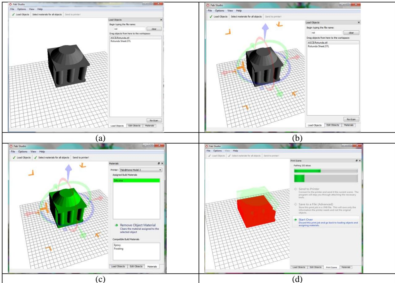
Figure 4: In order to use the new framework in FabStudio a user must load an object (a), position and scale it (b) assign a material to STL files or unmatched AMF files (c), and send to printer (d)
