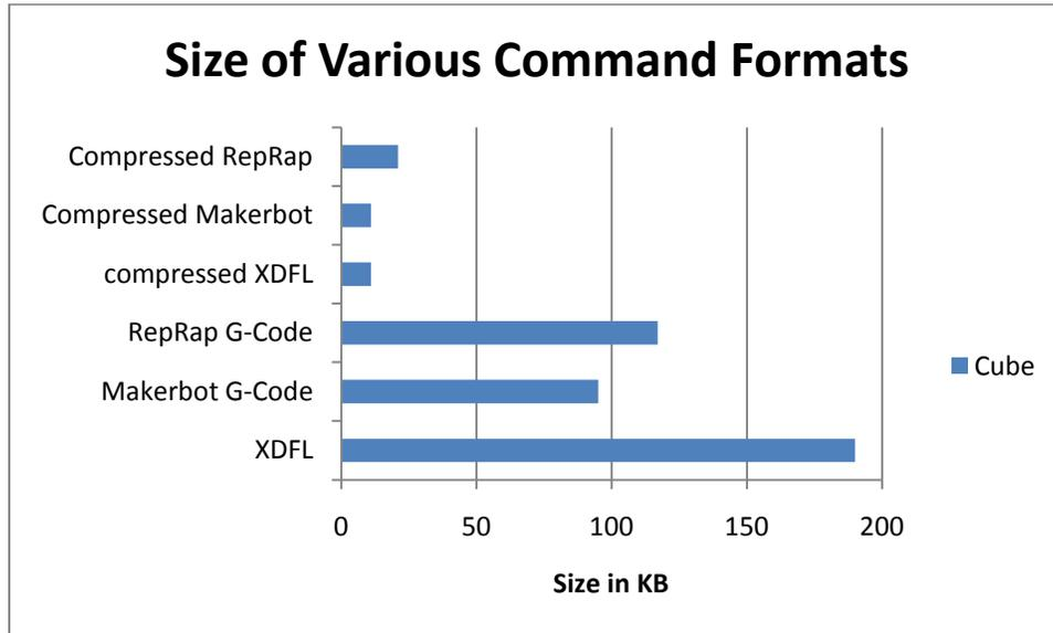
Figure 6: A comparison of XDFL verses two standard G-Code encodings for FDM
