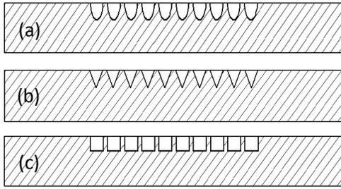
Figure 4 a) elliptical, b) triangular and c) rectangular flow fields with 10 passes.
