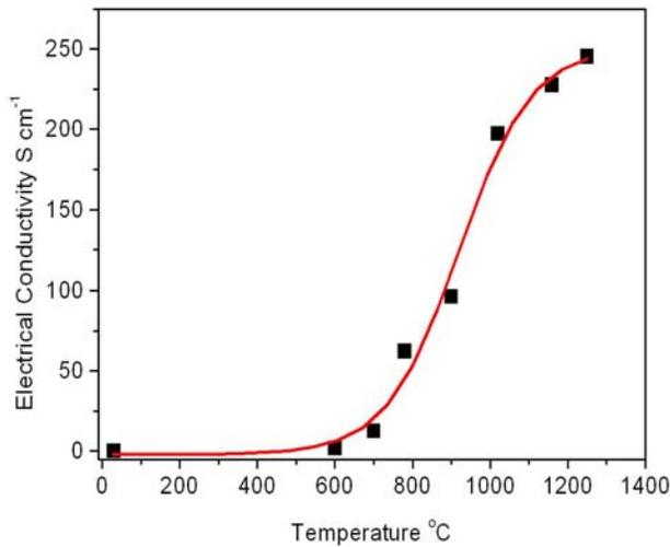
Figure 6 a) Electrical conductivity of graphite-phenolic parts w.r.t burnout temperature.
