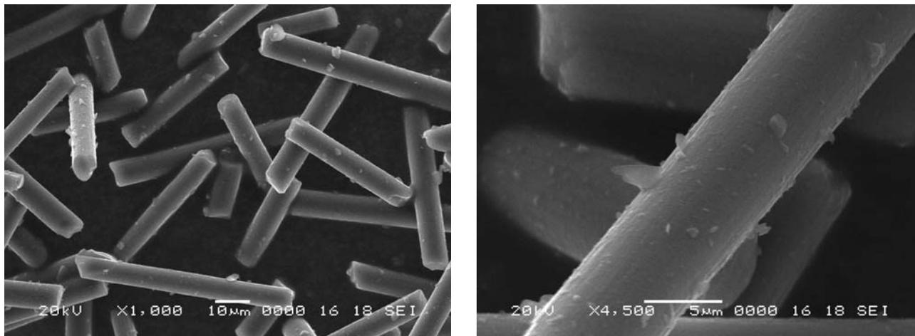
**Figure 3.** SEM images of the carbon fiber at a) 1000x and b) 4500x magnification.
