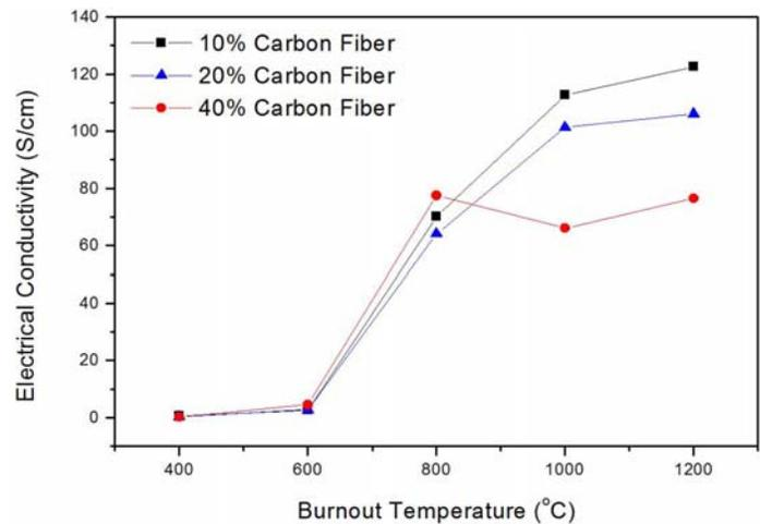
Figure 6 b) Electrical conductivity of carbon fiber added parts w.r.t burnout temperature.
