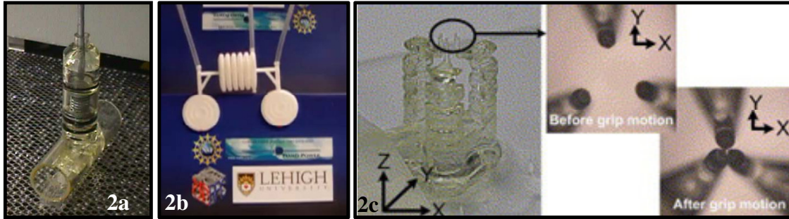
Figure 2. Fluid Power Actuators Grown Directly using Additive Manufacturing (2a-Wisner-2004, 2b-Zientarski-2009, 2c-Kang-2004).
