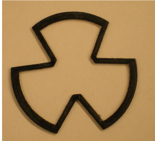
Figure 7: Seal Between Back Plate to Actuator Housing
